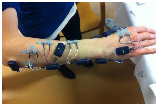
Fig1.1 Electrodes placed on the forearm, surface EMG.
