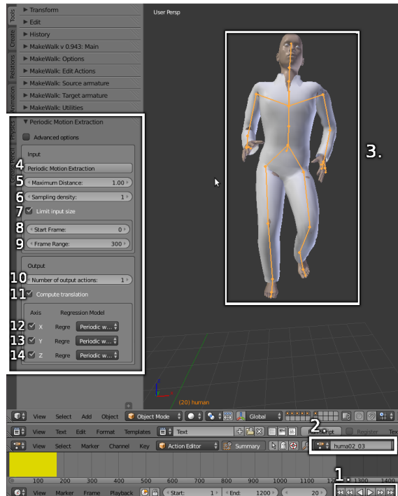
Figure 5.2: The figure shows the plugin interface and what it looks like when we mark an armature that which we wish to extract a periodic motion for when Object Mode is active.
