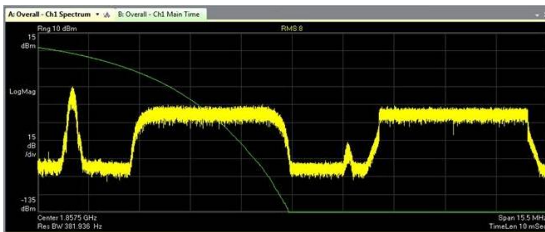
Figure 4-6: Spectrum of multiple radio standards in a 15.5 MHz range centered at 1.8575 GHz using the 89600 VSA software.
