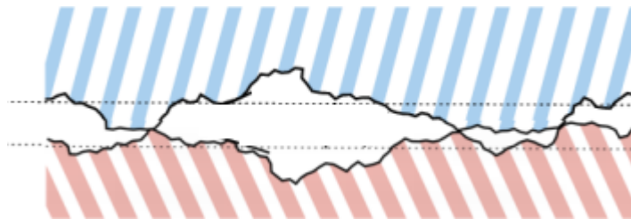
Figure 8: Shows in a microscopic level how the contact can be made in several points between the stator and frame[5].
