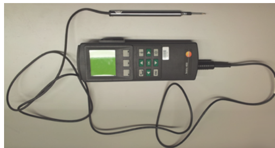
Figure 11: Testo 400 that was used for measuring air velocity
