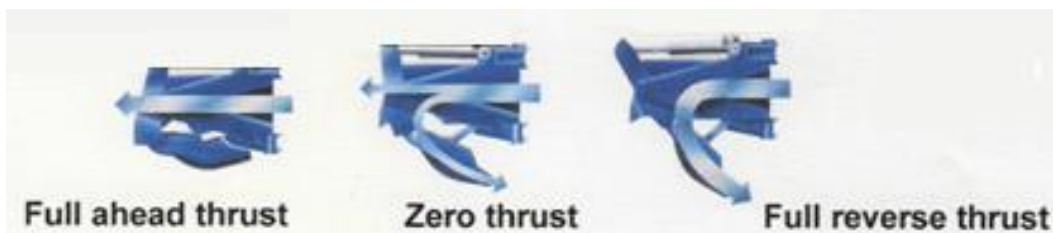
Fig 1.3c: Illustration of how the reversal mechanism redirects the jet stream from full ahead thrust, zero thrust to full reverse thrust. [1]
