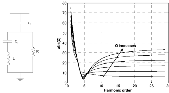
Figure 5.7: C-Type high-pass filter and its impedance curve [4]
