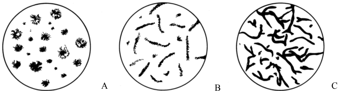
Figure 14, shows the different orientation for the graphite for SGI (A), CGI (B) and LGI (C), (ASM international, 1990).
