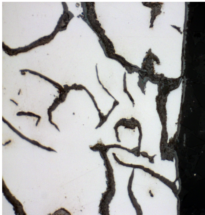
Figure 35, shows that the edge of a cross section of the stressed surface contains of several graphite particles.
