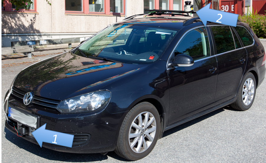
Figure 5.1. The test vehicle, showing the front-mounted automotive radar (1) and the roof-mounted LIDAR (2).
