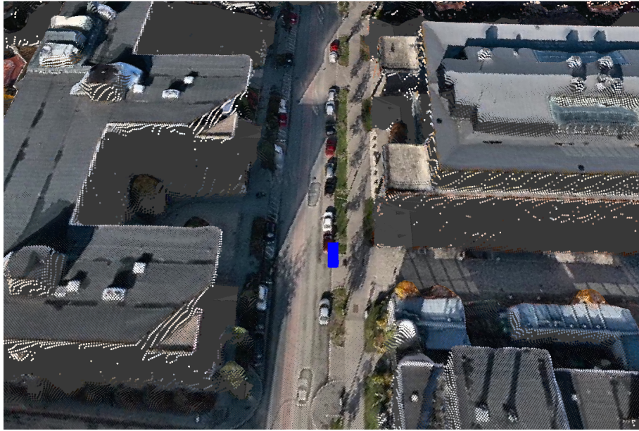
Figure 5.5. The graphical representation of the test vehicle showing the position with a 5 m bias, the upper interval of a D-GPS localization. The blue cuboid represents the ego-vehicle position.
