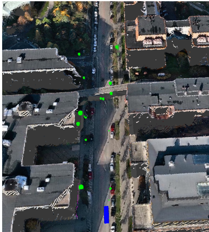
Figure 5.16. The system output of a typical use case. The blue cuboid shows the ego vehicle position, the green cylinders indicate radar obstacles and the purple dots indicate LIDAR measurements.
