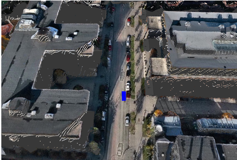
Figure 5.4. The graphical representation of the test vehicle showing the position with a 1 m bias, the lower interval of a D-GPS localization. The blue cuboid represents the ego-vehicle position.
