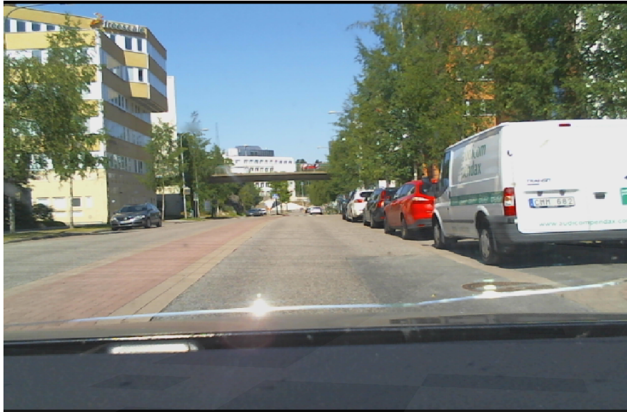
Figure 5.2. The on board camera of the test vehicle showing the reference position, i.e. that the test vehicle is positioned in the middle of the right lane.
