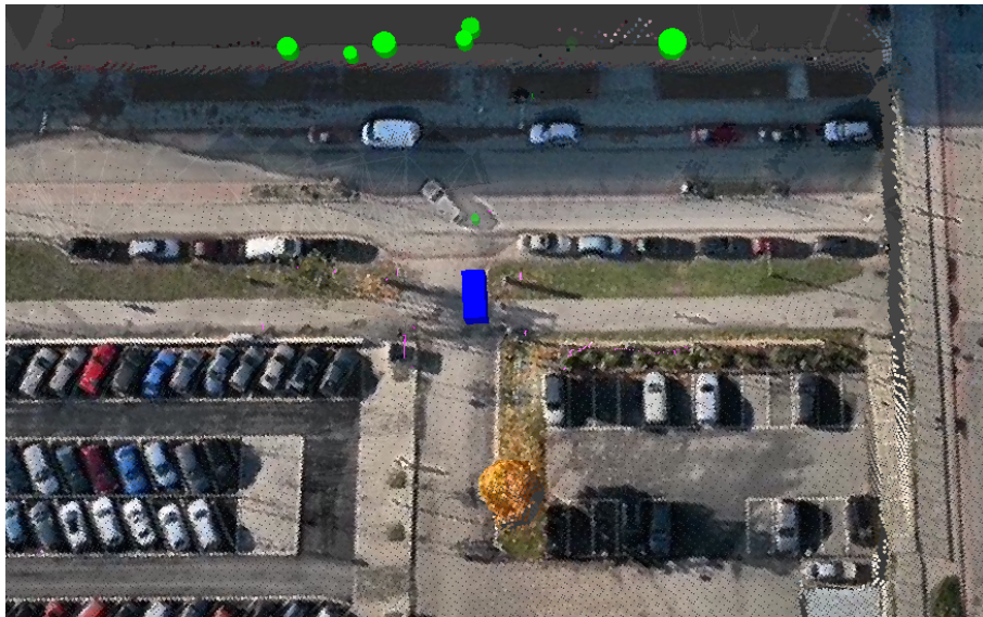
Figure 5.13. The system output as a vehicle is crossing ahead of the ego vehicle, straight in front of the ego vehicle. The blue cuboid shows the ego vehicle position, the green cylinders indicate radar obstacles and the purple dots indicate LIDAR measurements.
