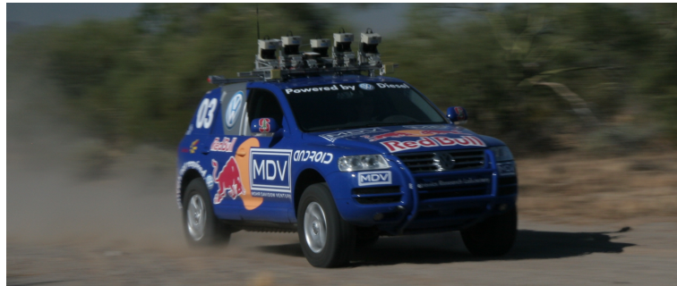
Figure 2.1. Stanley with the visible sensor platform, showing the roof mounted LIDARs [Woodward]
