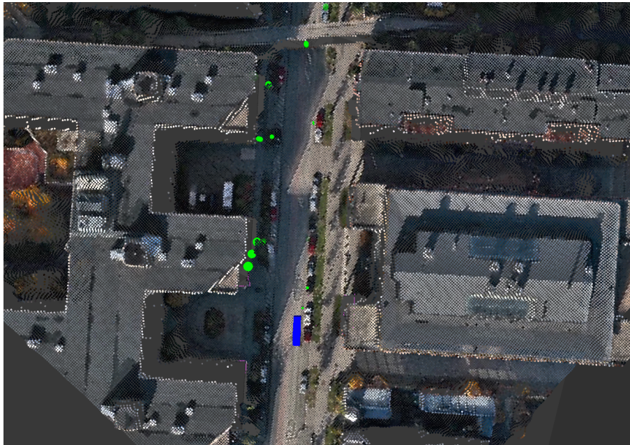
Figure 5.7. A 2D photo-realistic map with 0.5 m resolution. The blue rectangle represents the ego-vehicle position and the green circles represent identified obstacles.
