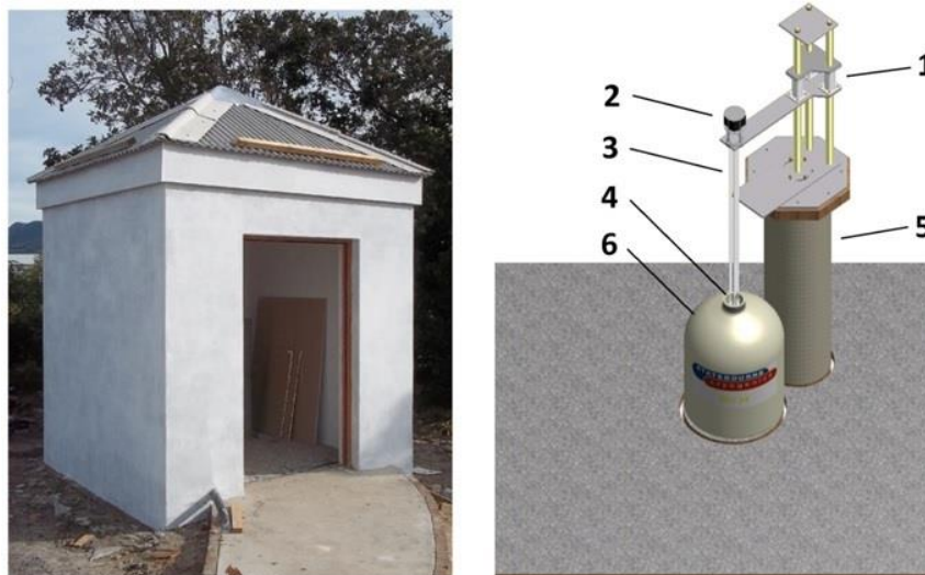
Figure 19: SQUID-hut and 3-axis SQUID system. (1) SQUID-lift; (2) PFLs; (3) Probes; (4) SQUIDS; (5) SQUID-lift pillar; (6) Dewar.
