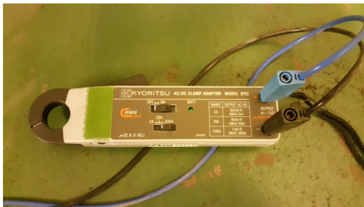
Figure 4.6: AC/DC Clamp Adaptor Used for Current Measurements.
