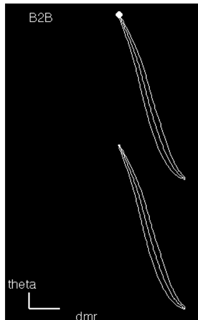
Figure 23: Altered, airfoil shape diffuser vane on a Blade to Blade (B2B) view.
