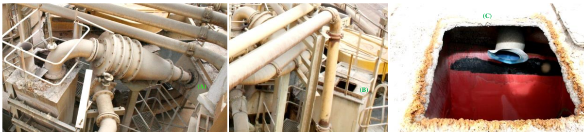
Figure 4-8: Illustration of fitting of; (A) the spigot onto the underflow box, (B) the underflow box opening and (C) the spigot seen from the opening
