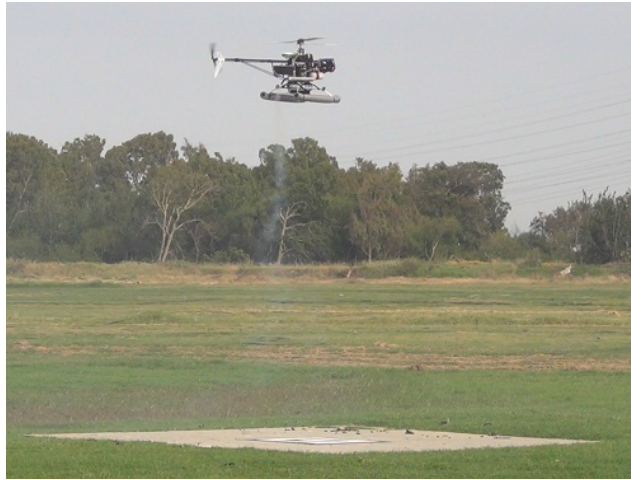
Figure 1.3: Autonomous landing of the X-Cell helicopter using monocular vision. Photo obtained from [3].
