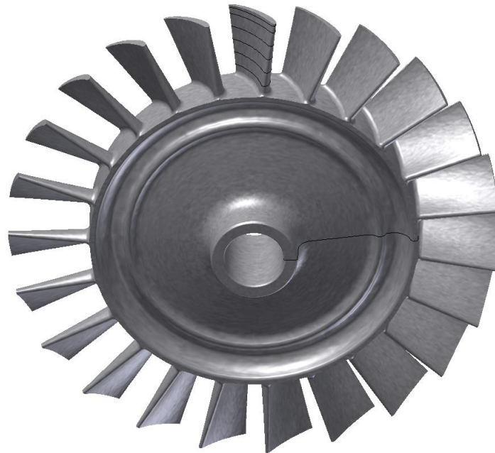
Figure 2-3: CMM measurement paths on the turbine rotor wheel
