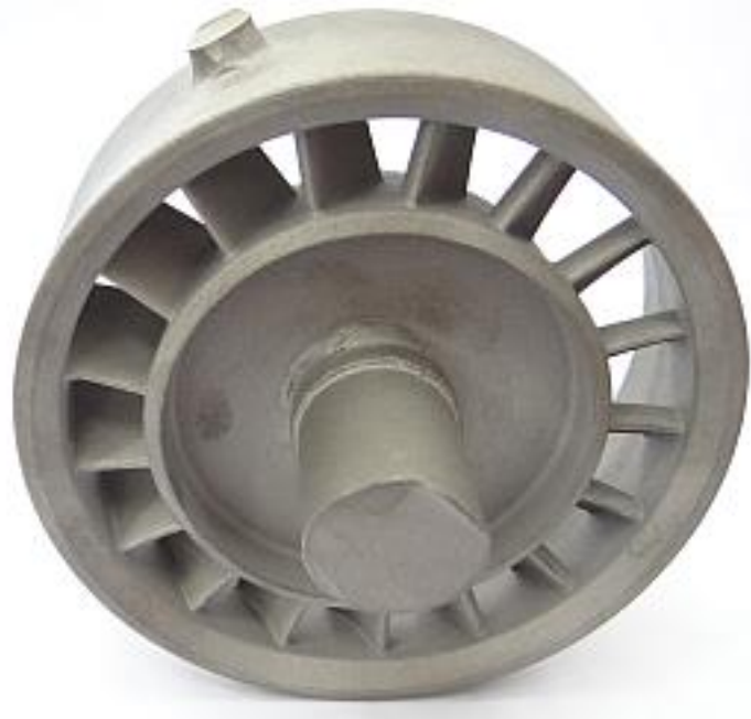
Figure 7-7: Stator casting made using a Solidscape 3Z Model pattern
