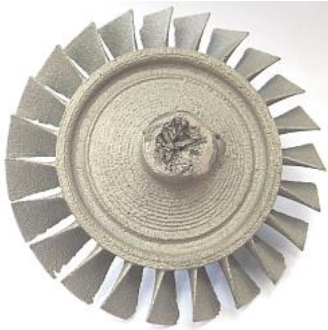
Figure 7-5: Rotor casting made using a PrimeCast 101 pattern
