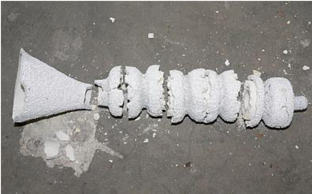
Figure 7-4: Ceramic mould destroyed by firing PrimeCast 101 stator patterns
