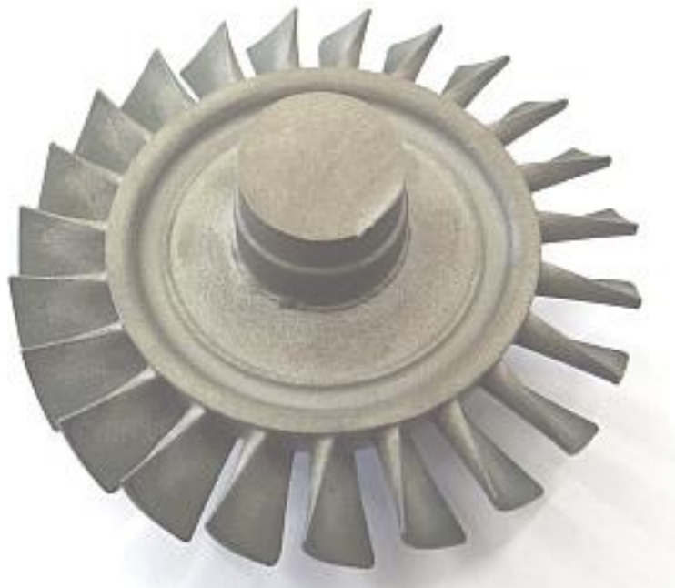
Figure 7-6: Rotor casting made using a Solidscape 3Z Model pattern
