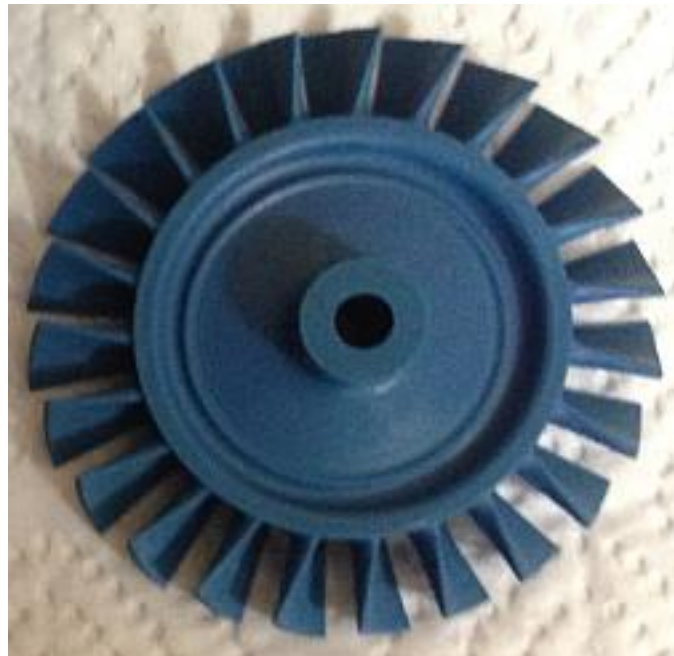
Figure 7-3: Solidscape 3Z Model rotor pattern
