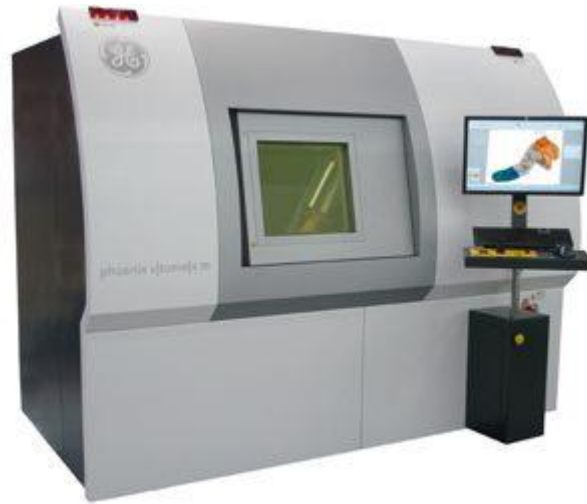
Figure 2-4: Phoenix v|tome|x m high resolution CT-scanner
