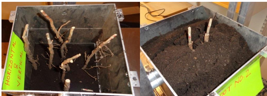
Figure 84 Roots inside the test box and soil after test with 2 roots in horizontal orientation
