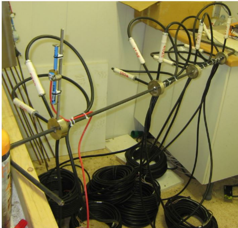
Figure 4.2: Strain gauges mounted on spiders on a rod. From Malm (2013b).
