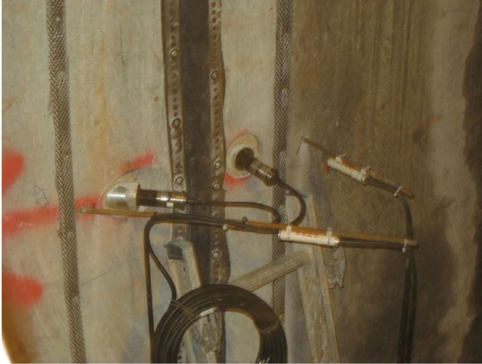
Figure 4.3: Strain gauges attached to reinforcement bars bolted into the rock. From Malm (2013b).
