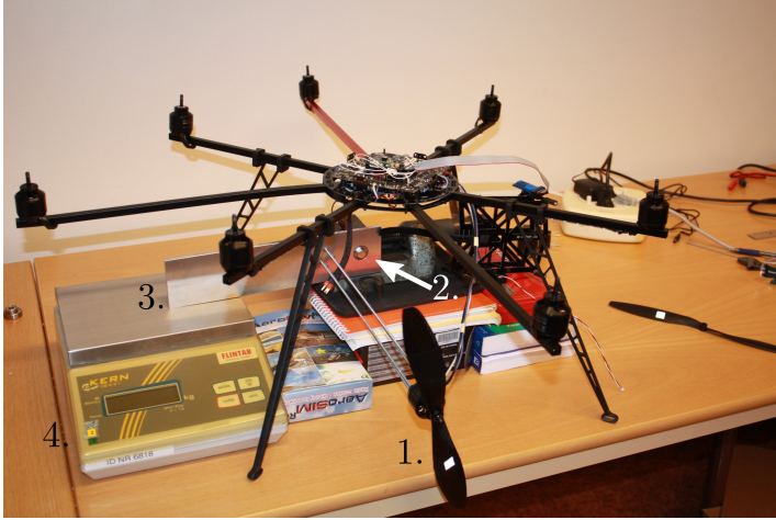
Figure 4.15: The test rig used in the first attempt to estimate the torque constant. The motor is placed horizontally (1), attached to a metallic plate (3) which can rotate around a ball bearing (2). The metallic plate is placed on a digital scale (4).
