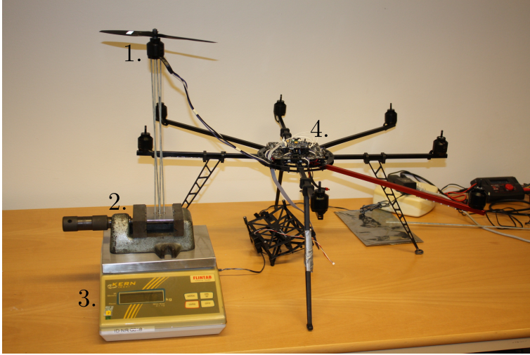
Figure 4.13: The test rig used to estimate the thrust constant including a motor unmounted from the platform (1), a vise (2), a digital balance scale (3) and the platform (4).
