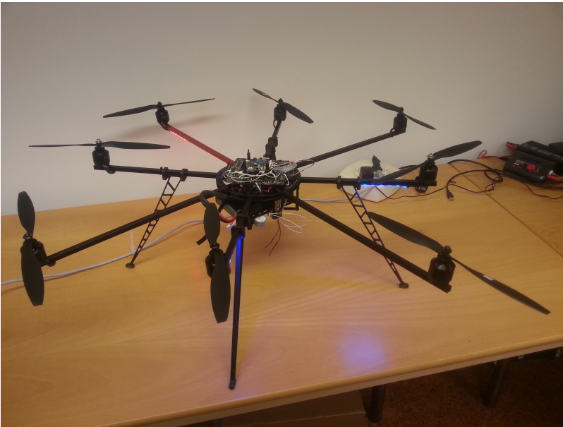
Figure 3.1: An overview of the octorotor platform. The front of the octorotor is distinguished by the red arm. The motors are mounted at the end of each arm. All avionics are mounted on the central plate.
