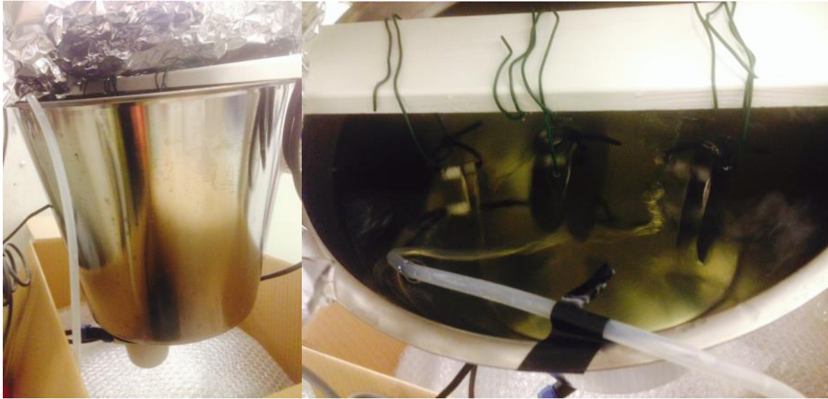
Figure 4-2: Arrangement for the ultrasound tests. On the left the ultrasound device can be seen attached to the bottom of the tank. On the right the plates and the tube from the aquarium pump can be seen.
