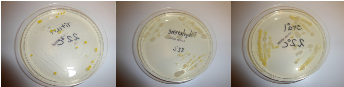
Figure C-4: The agar plates that swabbed the plates during ultrasound test. These plates had been incubated in room temperature for 9 days. The pictures are taken with a Sony Cyber-shot DSC- W290 camera.
