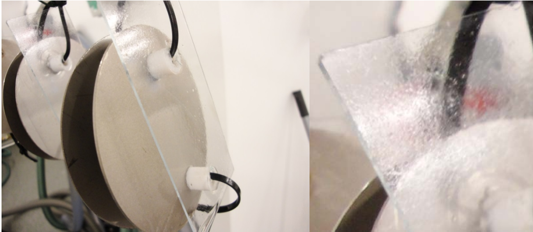
Figure B-1: Pictures taken from plates that had been immersed 10 days in the bucket when ultrasound not was operating. The second picture is a part of the first picture zoomed in. The pictures are taken with a Sony Cyber-shot DSC- W290 camera.
