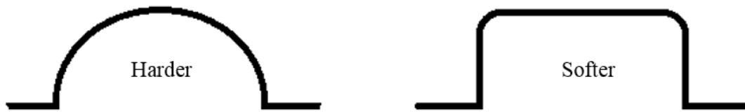
Figure 47 Schematic picture of the materials hardness effect on the contact area.
