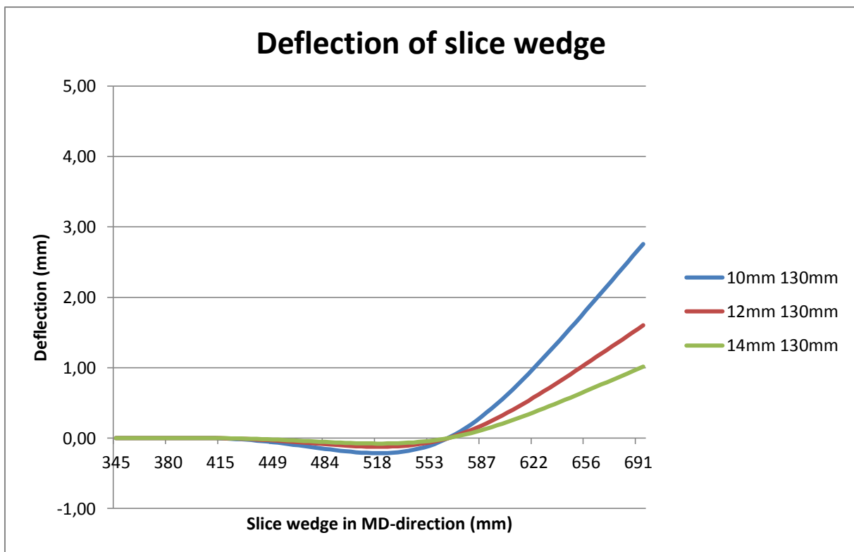
Figure 31 Deflection of the slice wedge with free length 130mm
