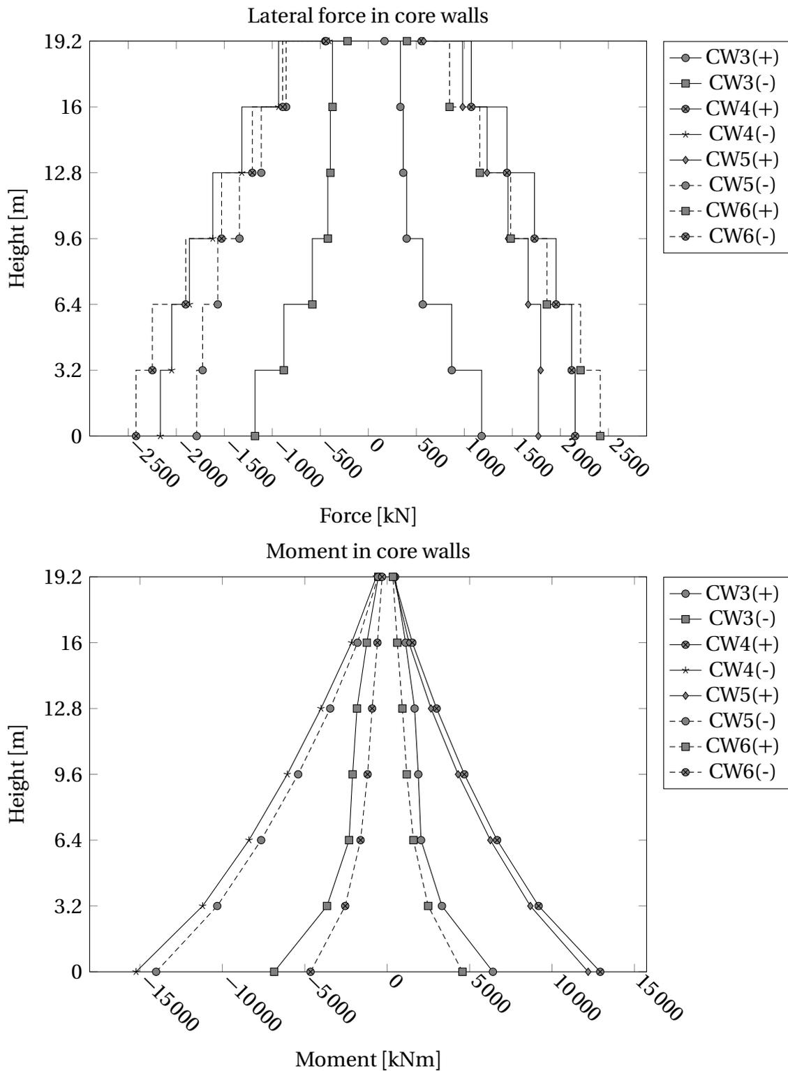
**Figure 5.10:** [Case 4:  $a_g \cdot S = 0.28 \text{ g}$ , DCL:  $q = 1.5$ ] Lateral force and moment in the core walls from analysis in RSA2014 ((+): positive sign seismic action, (-): negative sign seismic action).
