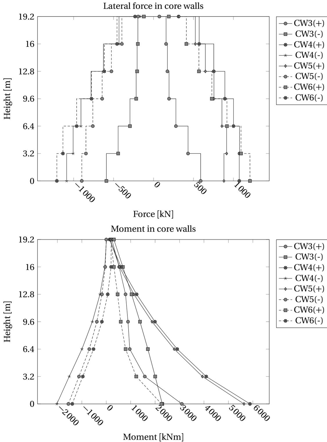
**Figure 5.11:** [Case 4:  $a_g \cdot S = 0.28 \text{ g}$ , DCM:  $q = 3.0$ ] Lateral force and moment in the core walls from analysis in RSA2014 ((+): positive sign seismic action, (-): negative sign seismic action).
