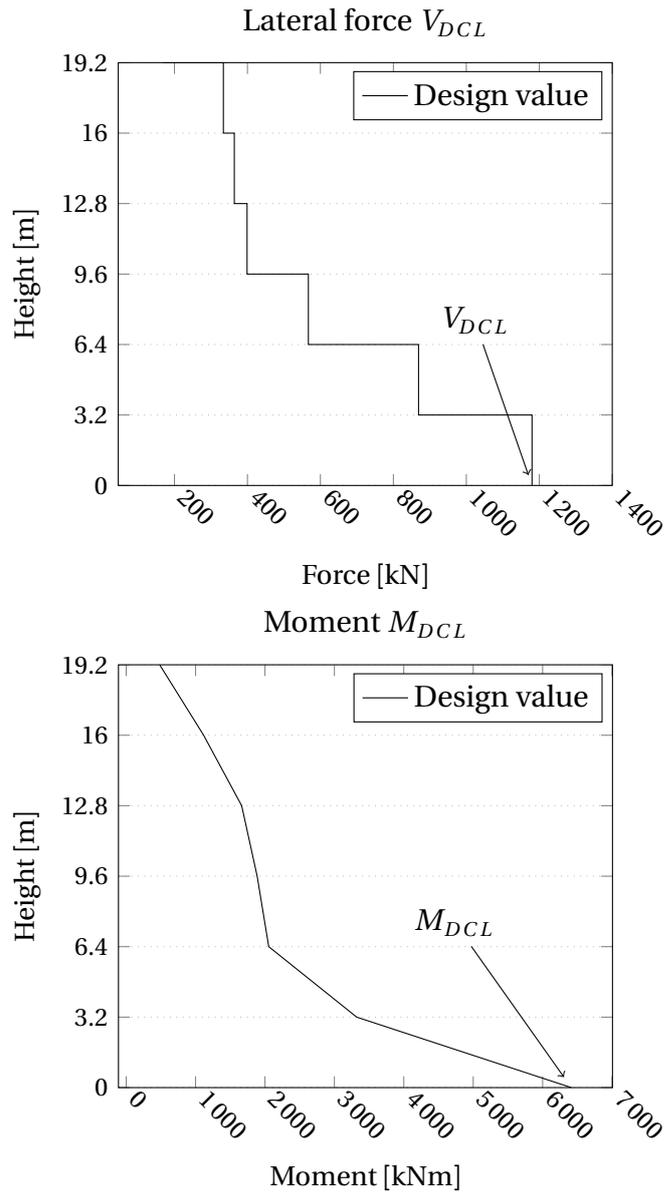
**Figure 5.13:** Lateral force and the moment in core wall 3 for DCL-design (Case 4:  $a_g = 0.28$  g).
