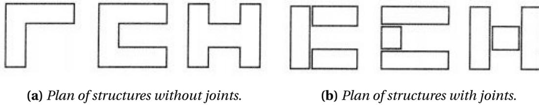
**Figure 4.2:** Division of structure into regular and simpler plans (Bachmann, 1997).
