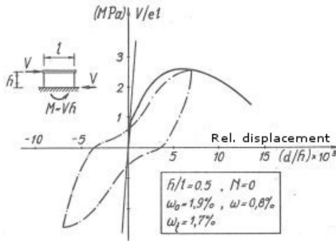
**Figure 3.14:** Wall failure mechanism due to dominating shear (Anastasiadis, 1989).
