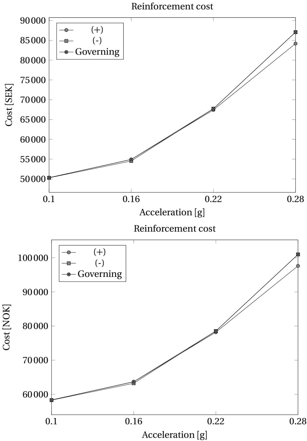
**Figure 5.16:** [DCM:  $q = 3.0$ ] Total cost development of reinforcement in DCM with increasing  $a_g \cdot S$ . (+) and (-) denotes positive respectively negative direction of seismic load in the load combination for analysis.
