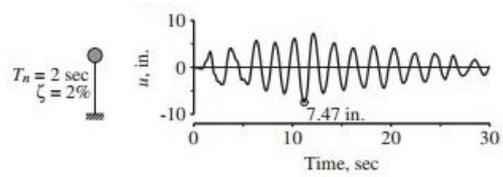
(d) Deformation time-history response of SDOF-system with  $T_n = 2\text{ s}$  and  $\zeta = 2\%$ .
