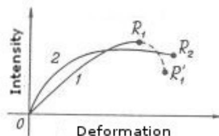
**Figure 3.4:** Ductile and brittle materials ( $R_1$ :Brittle  $R_2$ :Ductile) (Anastasiadis, 1989).
