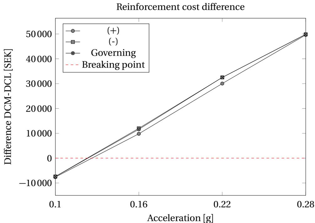
**Figure 5.18:** Difference between the total reinforcement costs for DCL- and DCM-design in Swedish kronor. (+) and (-) denotes positive respectively negative direction of seismic load in the load combination for analysis.
