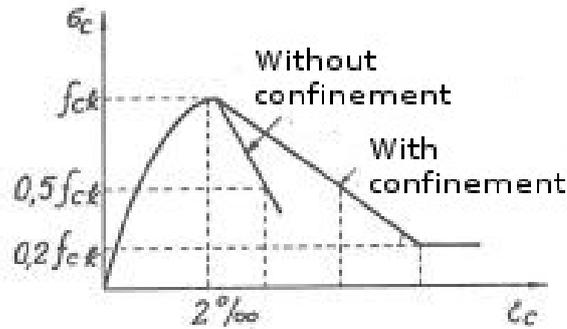
**Figure 3.7:** Enclosure of concrete (Anastasiadis, 1989).
