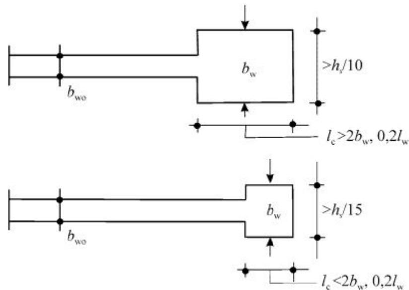
**Figure 4.8:** Minimum thickness of confined boundary elements (EN-1998-1:2004).
