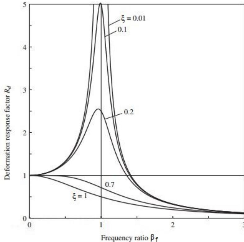
**Figure 3.25:** Deformation response factor for system excited by a harmonic force with changing excitation frequency  $\Omega$  (Chopra, 2007).
