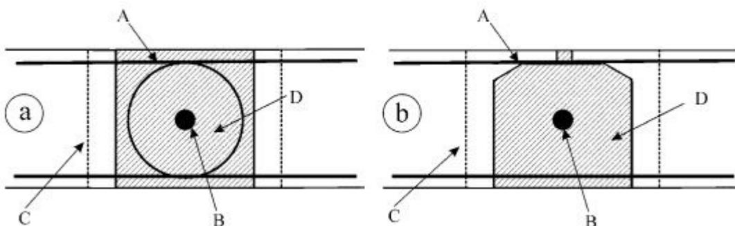
**Figure 4.13:** Cross-section of vertical connections between precast large-panels. A: reinforcement protruding across connection, B: reinforcement along connection, C: shear keys, D: grout filling space between panels (EN-1998-1:2004).
