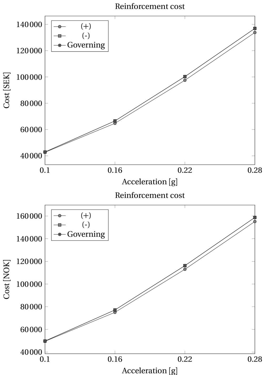
**Figure 5.15:** [DCL:  $q = 1.5$ ] Total cost development of reinforcement in DCL with increasing  $a_g \cdot S$ . (+) and (-) denotes positive respectively negative direction of seismic load in the load combination for analysis.
