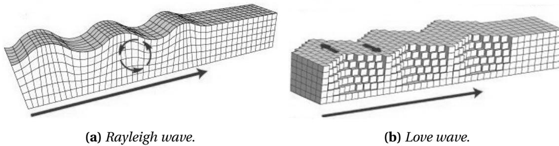
**Figure 2.8:** Propagation of surface waves through soil medium.
