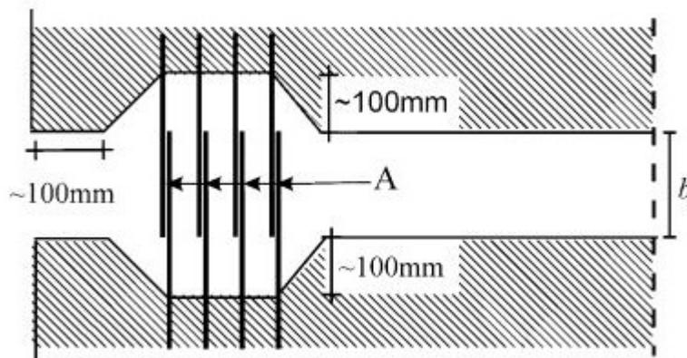
**Figure 4.12:** Tensile reinforcement possibly needed at the edge of walls. A: lap-welding of bars (EN-1998-1:2004).
