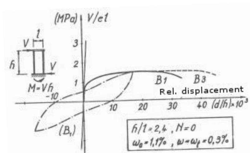
**Figure 3.11:** Wall failure mechanism due to dominating bending (B1:  $\mu = 30$  B2:  $\mu > 30$ ) (Anastasiadis, 1989).
