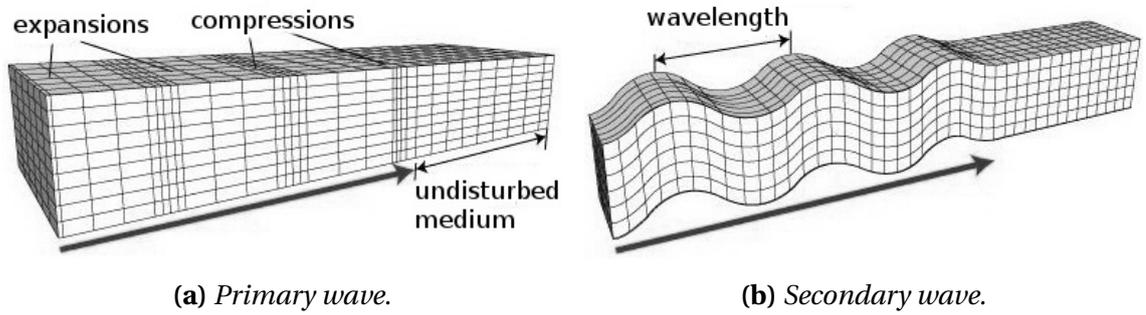
**Figure 2.7:** Propagation of body waves through soil medium.
