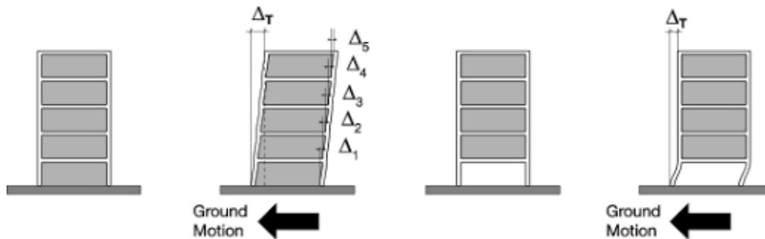
**(a)** Distributed ductile behaviour in connections.
