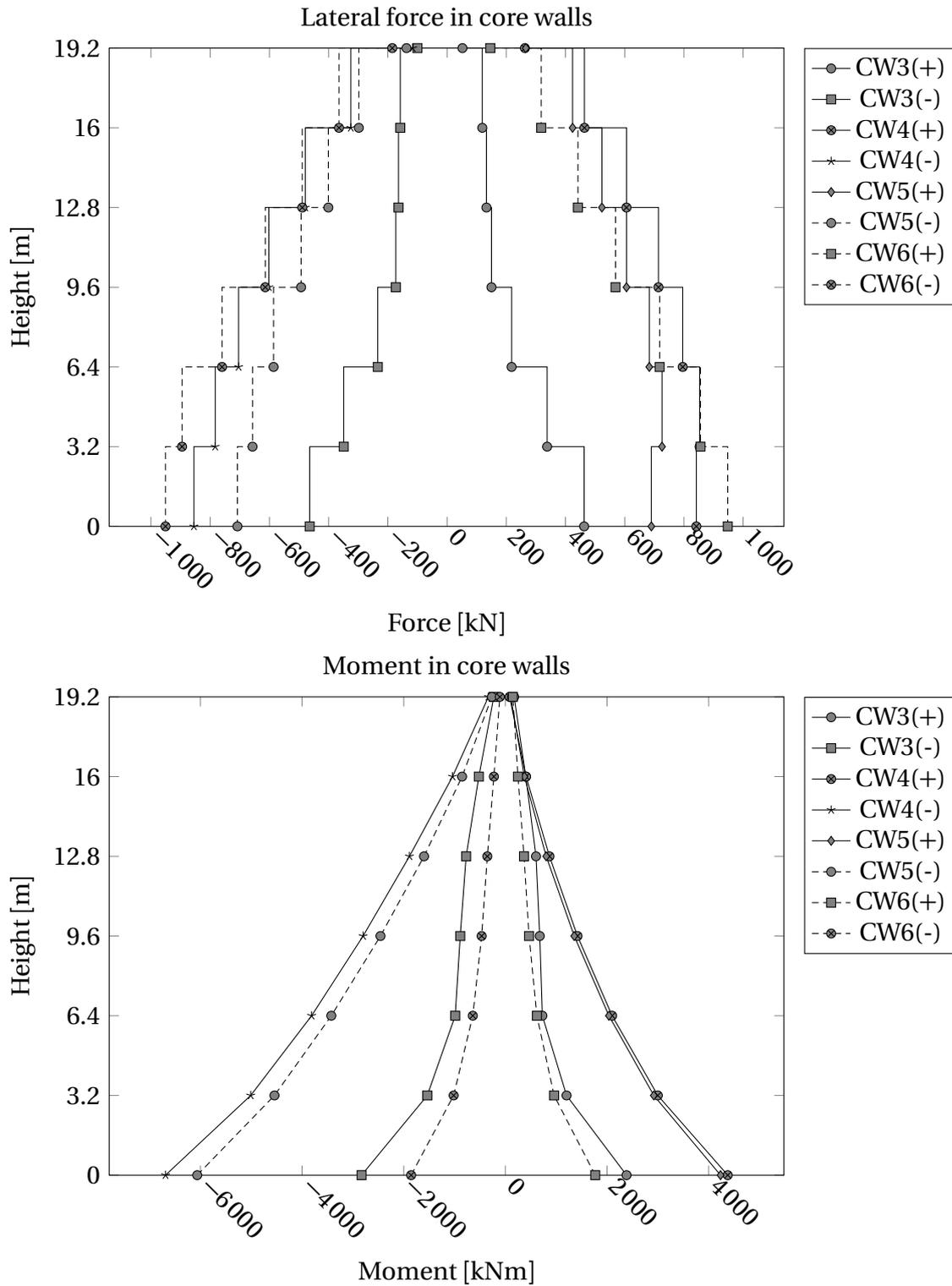
**Figure 5.9:** [Case 3:  $a_g \cdot S = 0.22 \text{ g}$ , DCM:  $q = 3.0$ ] Lateral force and moment in the core walls from analysis in RSA2014 ((+): positive sign seismic action, (-): negative sign seismic action).
