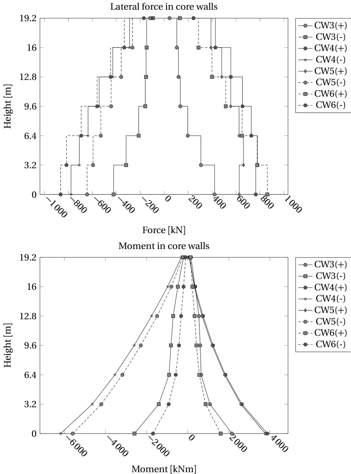
**Figure 5.4:** [Case 1:  $a_g \cdot S = 0.10 g$ , DCL:  $q = 1.5$ ] Lateral force and moment in the core walls from analysis in RSA2014 ((+): positive sign seismic action, (-): negative sign seismic action).
