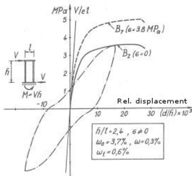
**Figure 3.12:** Wall failure mechanism due to dominating shear (Anastasiadis, 1989).
