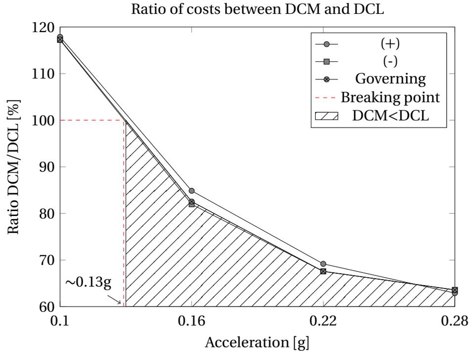
**Figure 5.17:** Ratio of total reinforcement costs in DCL- and DCM-design. (+) and (-) denotes positive respectively negative direction of seismic load in the load combination for analysis.
