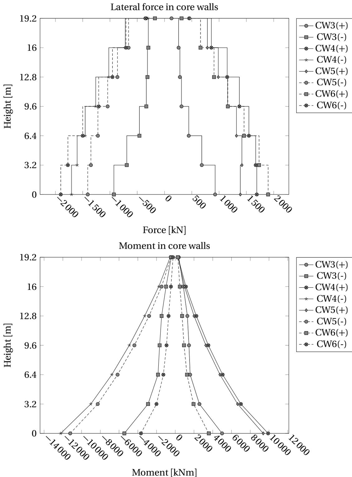
**Figure 5.8:** [Case 3:  $a_g \cdot S = 0.22$  g, DCL:  $q = 1.5$ ] Lateral force and moment in the core walls from analysis in RSA2014 ((+): positive sign seismic action, (-): negative sign seismic action).
