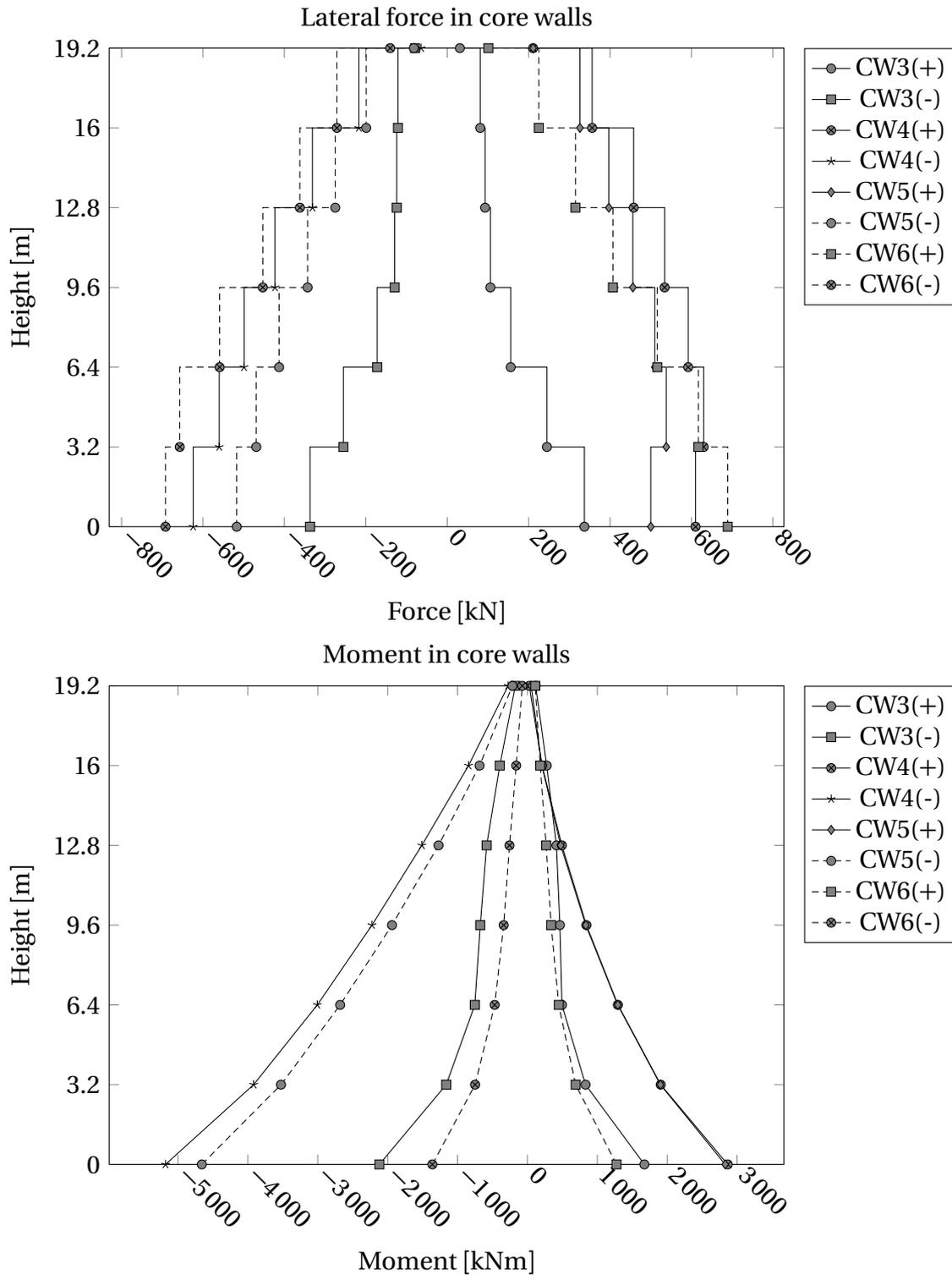
**Figure 5.7:** [Case 2:  $a_g \cdot S = 0.16$  g, DCM:  $q = 3.0$ ] Lateral force and moment in the core walls from analysis in RSA2014 ((+): positive sign seismic action, (-): negative sign seismic action).
