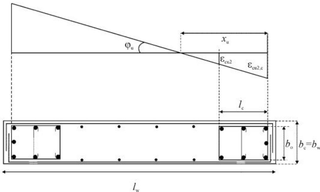
**Figure 4.11:** Confined boundary element of free-edge wall end (EN-1998-1:2004).
