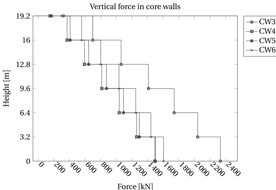
**Figure 5.12:** Vertical static force from analysis in RSA2014.
