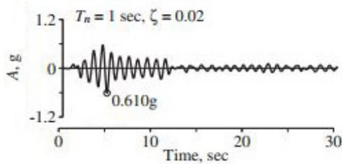
(c) Pseudo-acceleration response of SDOF-system to El Centro ground motion ( $T_n = 1$  s and  $\zeta = 2\%$ ).
