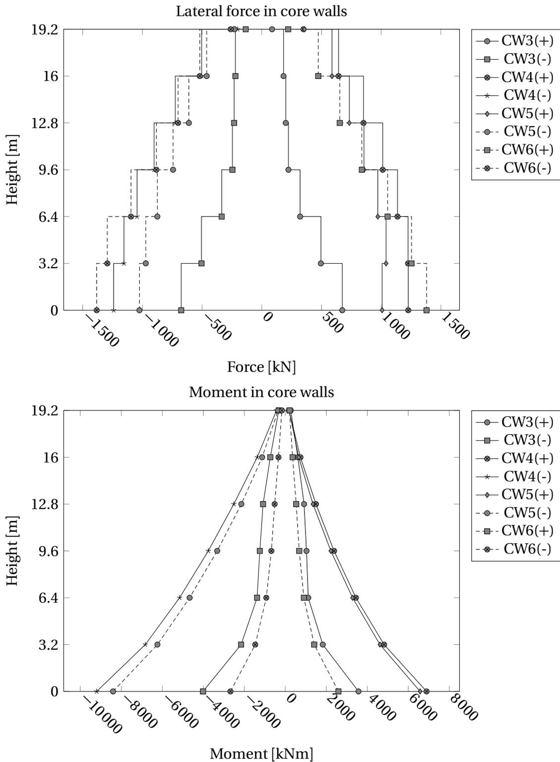
**Figure 5.6:** [Case 2:  $a_g \cdot S = 0.16$  g, DCL:  $q = 1.5$ ] Lateral force and moment in the core walls from analysis in RSA2014 ((+): positive sign seismic action, (-): negative sign seismic action).
