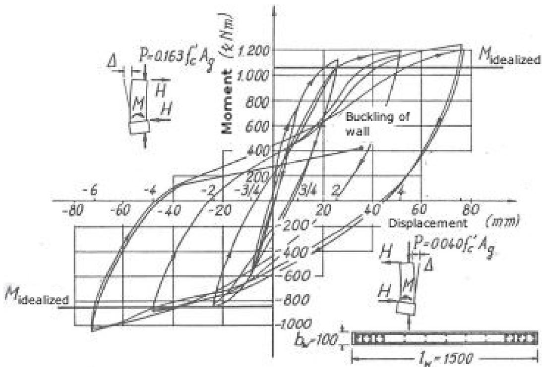
**Figure 3.15:** Wall failure mechanism due to dominating shear (Anastasiadis, 1989).
