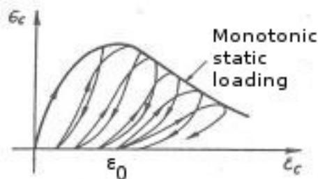
**Figure 3.6:** Cyclic compression of concrete (Anastasiadis, 1989).
