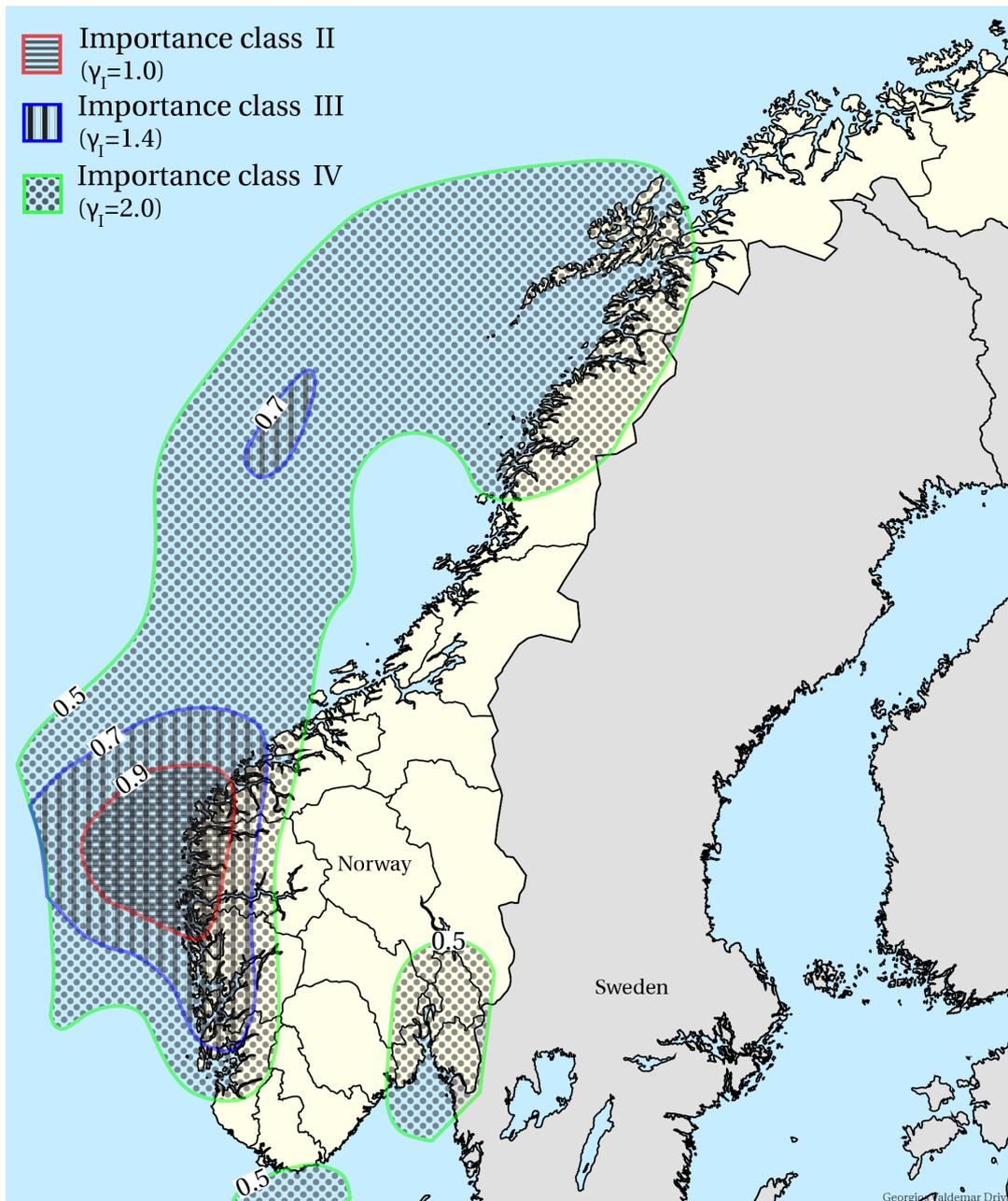
**Figure 5.20:** Regions in Norway where DCM-design is more cost efficient than DCL-design. The illustration is based on the Norwegian seismic zones represented Figure 4.4 and the results listed in Tables 5.12–5.14 referring to the seismic hazard parameter  $a_{g40Hz}$  [m/s<sup>2</sup>].
