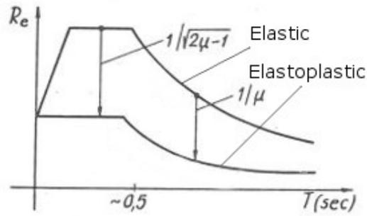
**Figure 3.33:** Elastic and inelastic acceleration response spectra (Anastasiadis, 1989).
