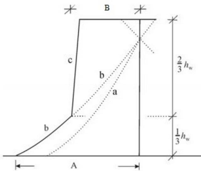
**Figure 4.10:** Design envelope of the shear forces in the walls of a dual system. *a* is the shear diagram from analysis, *b* is the magnified shear diagram, *c* is the design envelope, *A*:  $V_{wall,base}$  and *B*:  $V_{wall,top} \geq V_{wall,base}/2$  (EN-1998-1:2004).
