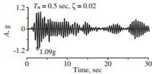
(b) Pseudo-acceleration response of SDOF-system to El Centro ground motion ( $T_n = 0.5$  s and  $\zeta = 2\%$ ).
