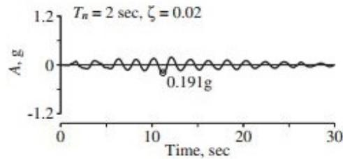
(d) Pseudo-acceleration response of SDOF-system to El Centro ground motion ( $T_n = 2$  s and  $\zeta = 2\%$ ).
