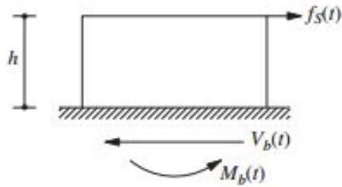
(a) Engineering response quantities: moment at base, shear force at base and equivalent static force.
