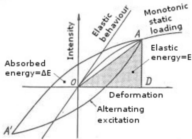
**Figure 3.2:** Calculation of the damping ratio (Anastasiadis, 1989).
