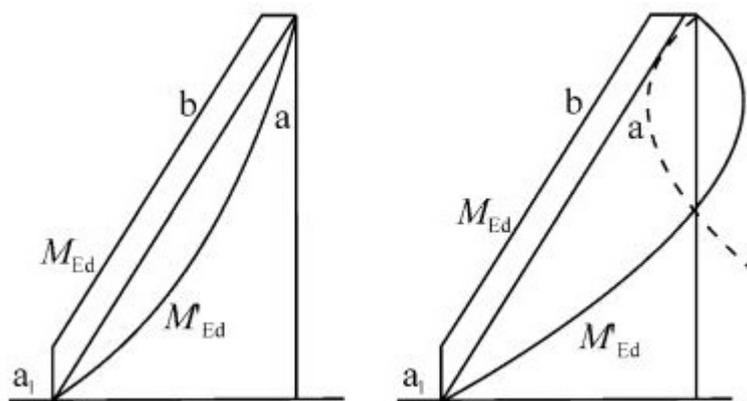
**Figure 4.9:** Design envelope for bending moments in slender walls. *a* is the moment diagram from analysis, *b* is the design envelope and  $a_1$  is the tension shift. (left: wall systems; right: dual systems) (EN-1998-1:2004).
