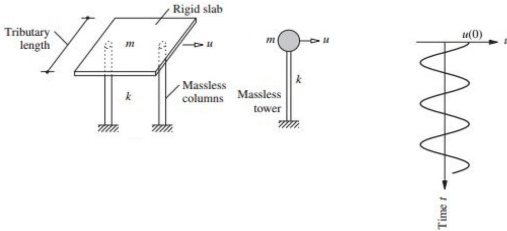
(a) Idealized pergola. (b) Idealized water tank. (c) Free vibration due to initial displacement  $u(0)$ .
