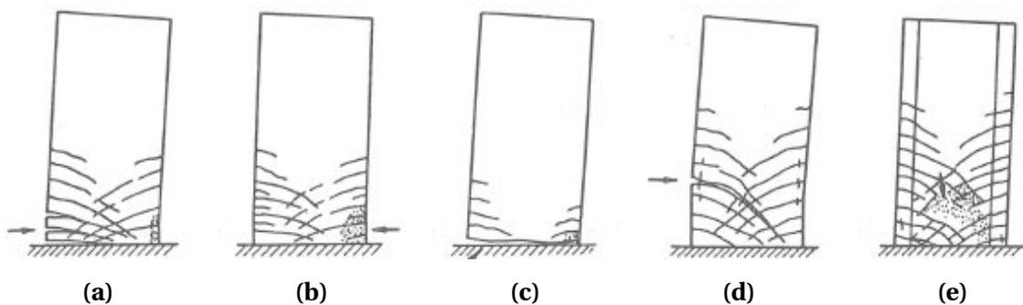
**Figure 3.10:** Wall failure mechanisms. (a) Yielding of reinforcement in tension. (b) Rupture of concrete in compression. (c) Fracture of reinforcement. (d) Yielding of longitudinal and transverse reinforcement. (e) Rupture of body-concrete (Anastasiadis, 1989).
