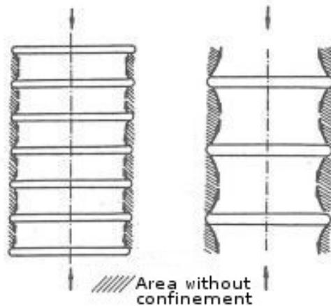
**Figure 3.8:** Affection of distance of transverse reinforcement (Anastasiadis, 1989).
