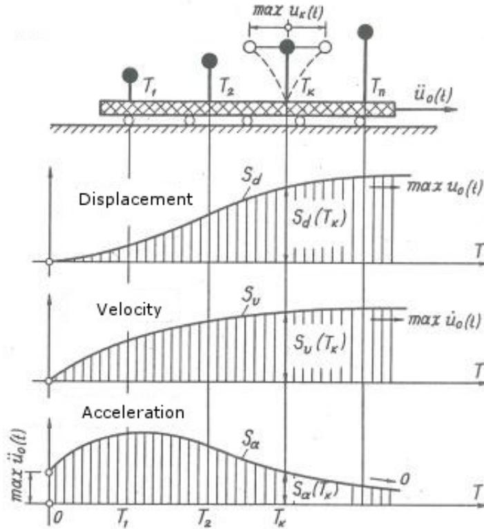
**Figure 3.27:** Generation of response spectrum based on seismic excitation (Anastasiadis, 1989).
