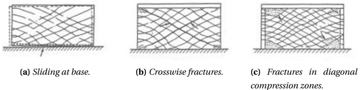
**Figure 3.13:** Wall failure mechanism of short walls (Anastasiadis, 1989).
