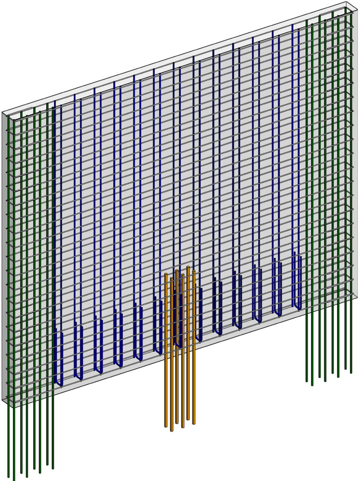
**Figure 5.21:** Schematic detailing of core wall in 3D.
