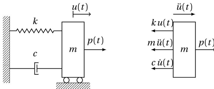
**Figure 3.18:** Free body diagram of single-degree-of-freedom system.
