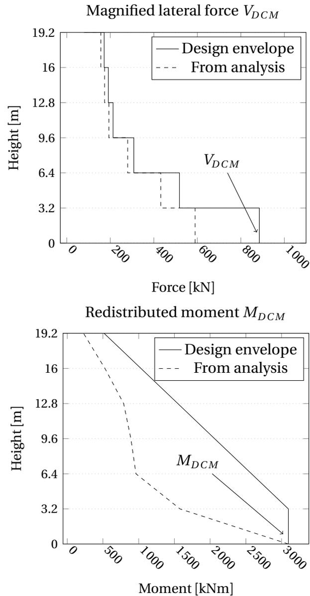
**Figure 5.14:** Design envelope of the lateral force and the moment in core wall 3 for DCM-design (Case 4:  $a_g = 0.28$  g).
