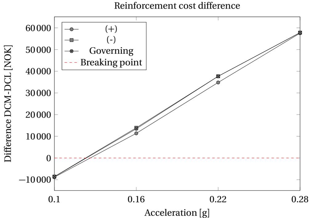
**Figure 5.19:** Difference between the total reinforcement costs in DCL- and DCM-design for Norwegian kroner. (+) and (-) denotes positive respectively negative direction of seismic load in the load combination for analysis.
