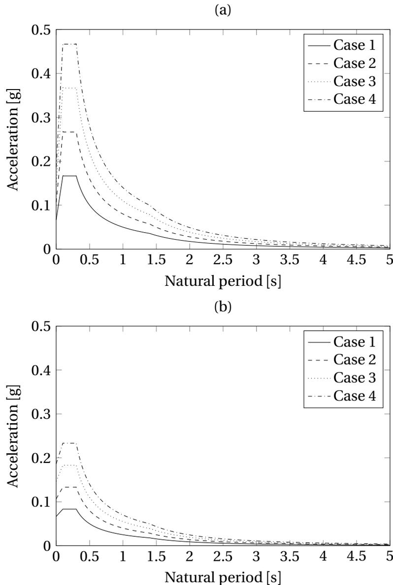
**Figure 5.3:** Design response spectra for analysis in RSA2014: (a) DCM-design (b) DCL-design (see Table 5.6).
