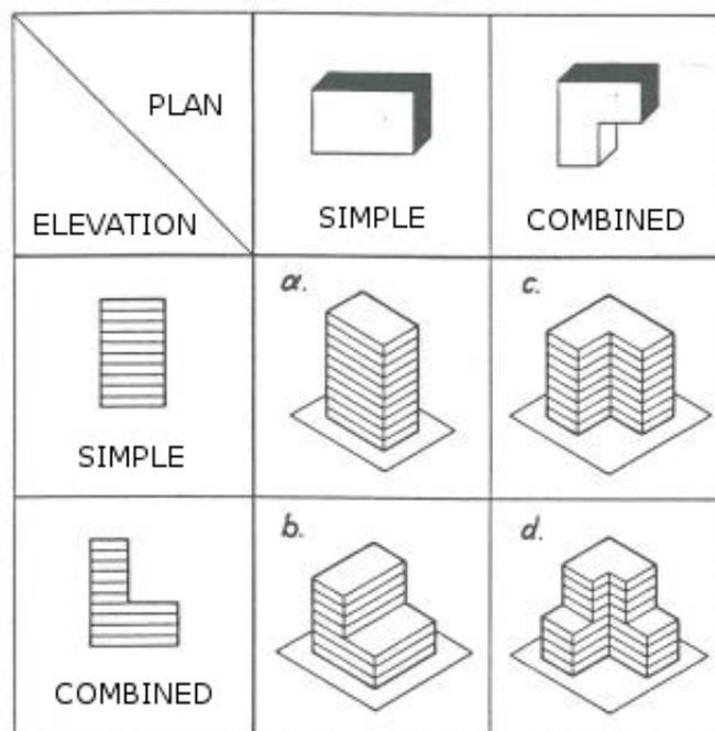
**Figure 4.6:** Illustration of structural layouts (Anastasiadis, 1989).
