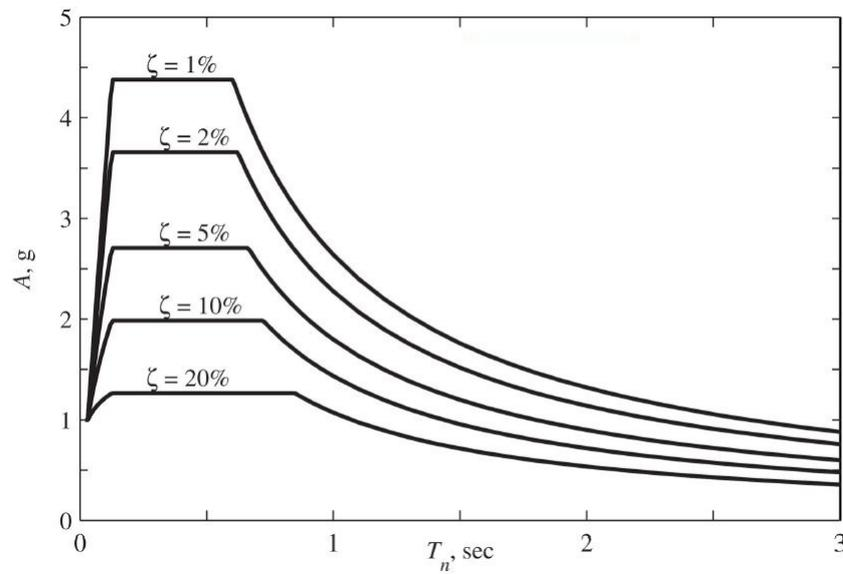
**Figure 3.30:** Damping effect on spectral pseudo-acceleration (Stojadinovic, 2013).
