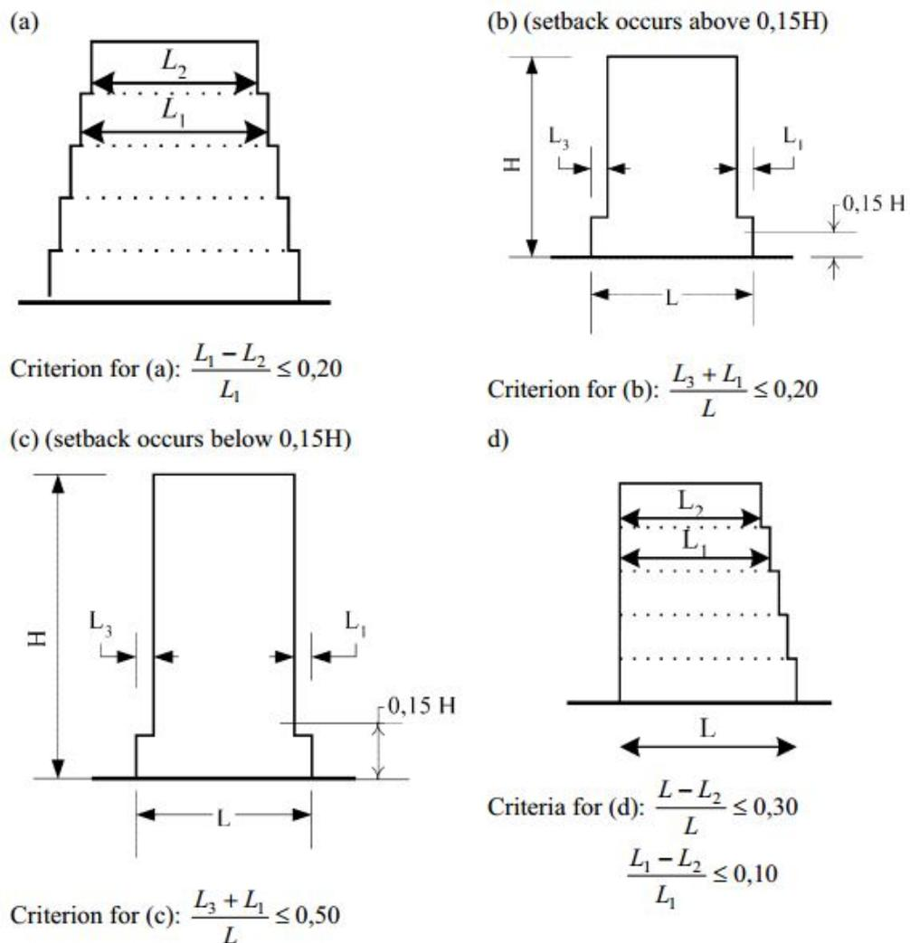
**Figure 4.7:** Criteria for regularity if setbacks in elevation (EN-1998-1:2004).
