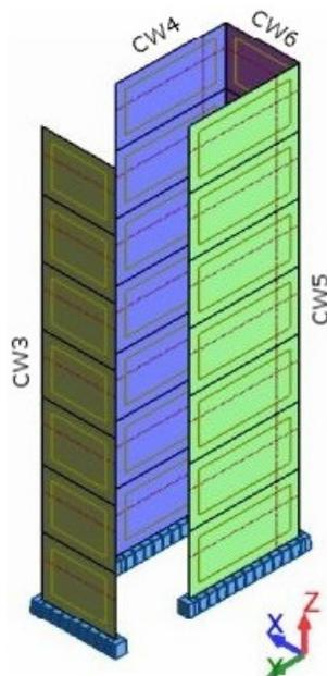
**Figure 5.2:** Core walls (linear releases marked with dotted lines).
