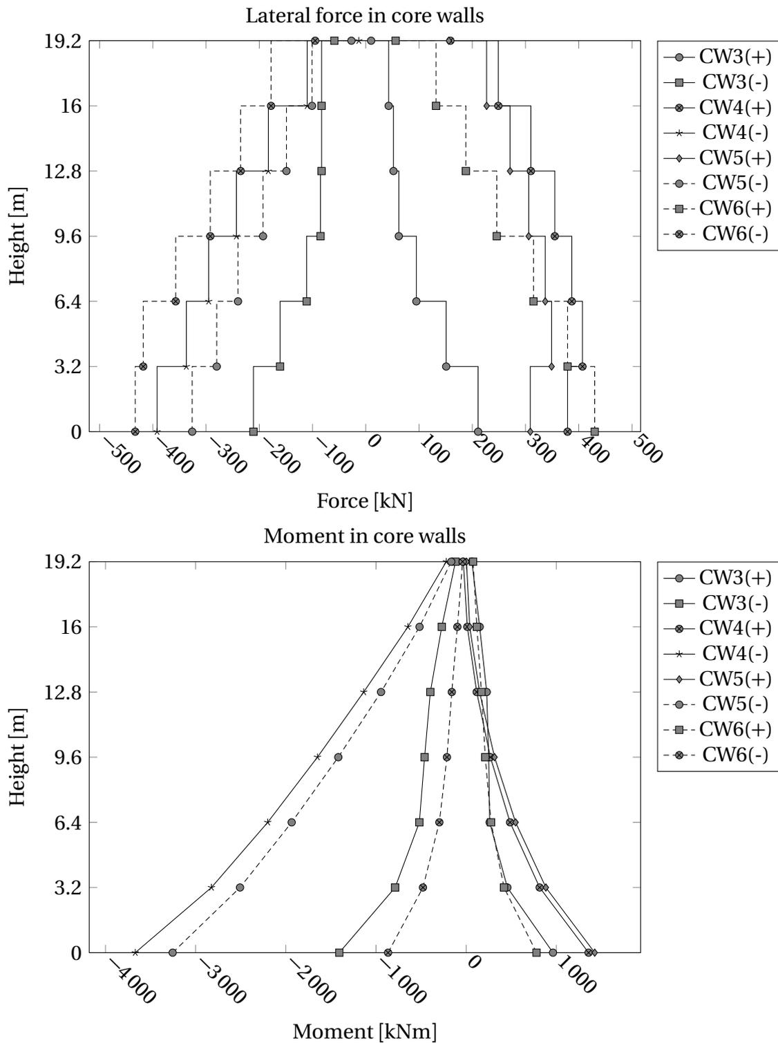
**Figure 5.5:** [Case 1:  $a_g \cdot S = 0.10 \text{ g}$ , DCM:  $q = 3.0$ ] Lateral force and moment in the core walls from analysis in RSA2014 ((+): positive sign seismic action, (-): negative sign seismic action).
