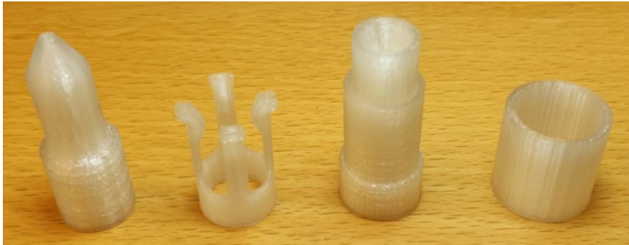
Figure 36. 3D-printed parts of the snap-fit concept. From left to right: electrode carrier, snap-carrier, driving shaft, spring biased socket.
