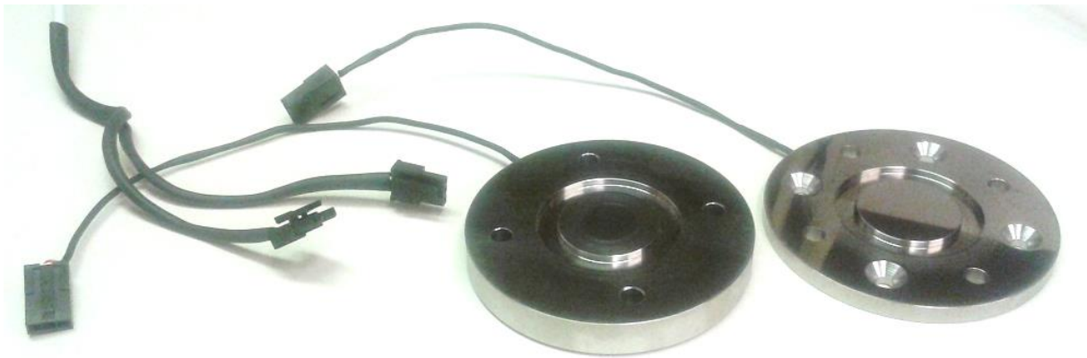
Figure 21. Temperature sensors in the upper and lower plates.
