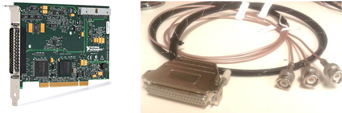
Figure 36. DAQ-Card: PCI6221 and the custom-made Dsub connector.
