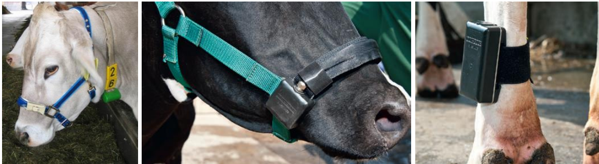
Figure 3-4. The MSR-ART rumination sensor (msr.ch). Figure 3-5. The RumiWatch NBS (rumiwatch.ch). Figure 3-6. The RumiWatch pedometer (rumiwatch.ch).
