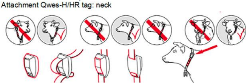
Figure 6-1. Mounting instructions for the Lely Qwes-H/HR tag (lely.com).
