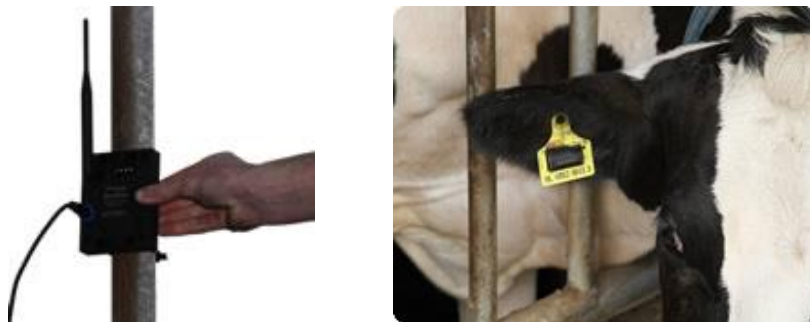
Figure 3-7. The SensOor system coordinator (cowmanager.com). Figure 3-8. The SensOor ear tag chip (cowmanager.com).
