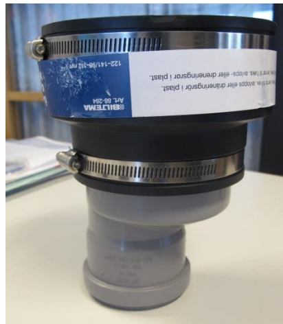
Figure 26. The reducer mounted in Odomin to create a greater splash.
