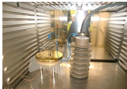
Figure 3.3: Brass electrodes connected to the insulator
