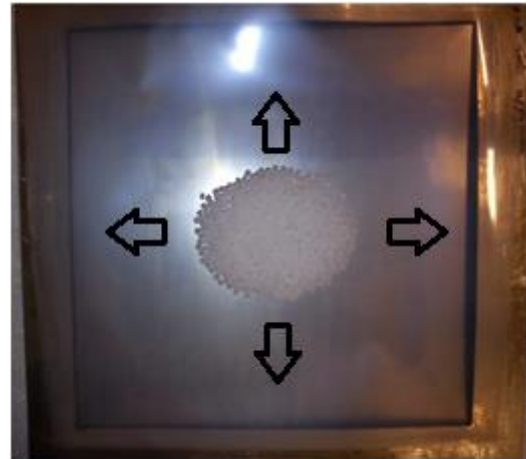
Figure 4.3: When the press is pressing shall it move the mould out in all directions whereas it also presses the air out to prevent voids
