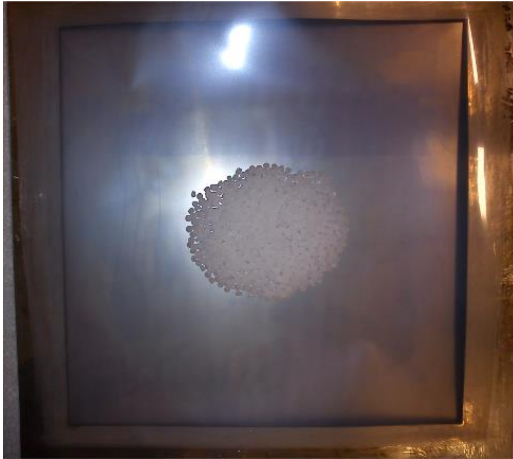
Figure 4.2: Mylar film covers the frame and the pellets gathered in the middle
