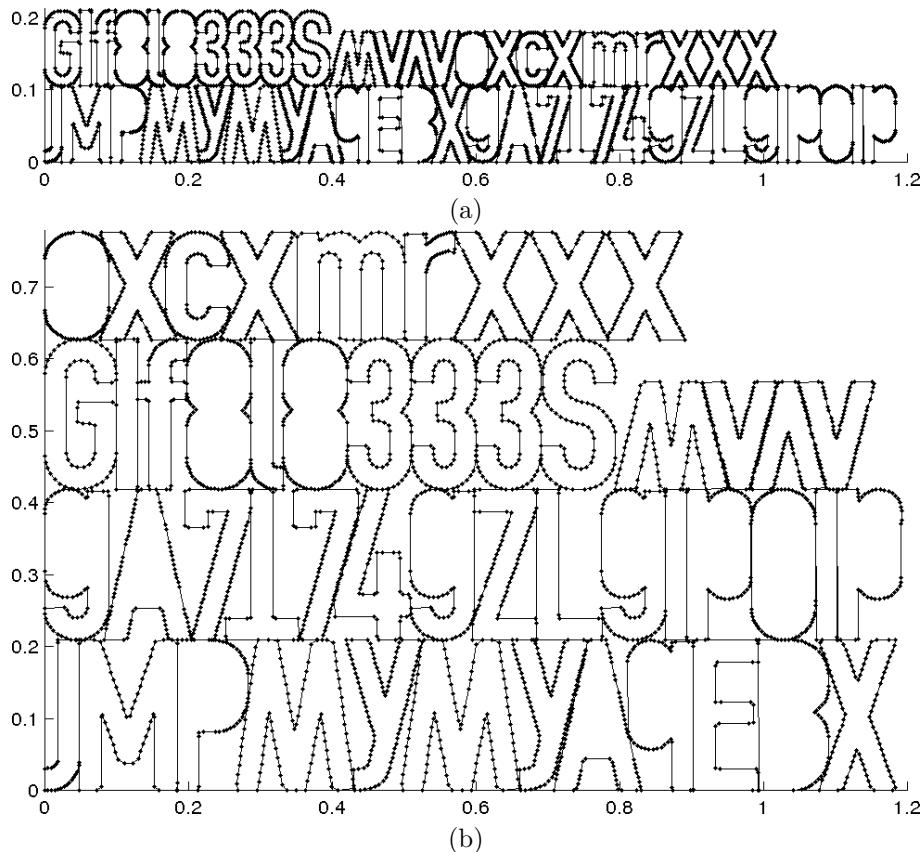
FIGURE 5.8: Example packings for the same set of items where rotations are allowed, with text heights of 105mm (a) and 210mm (b) respectively.
