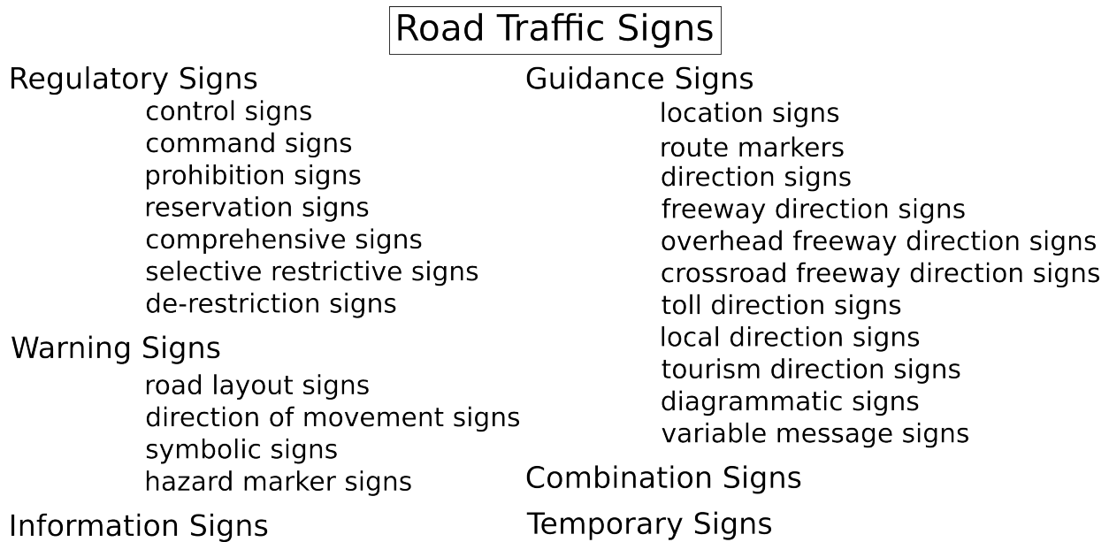
FIGURE 1.4: List of road traffic signs.
