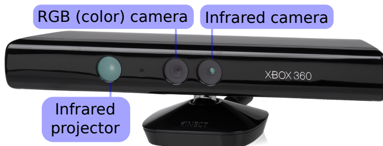
Figure 1.7: Microsoft Kinect structured light sensor [1]
