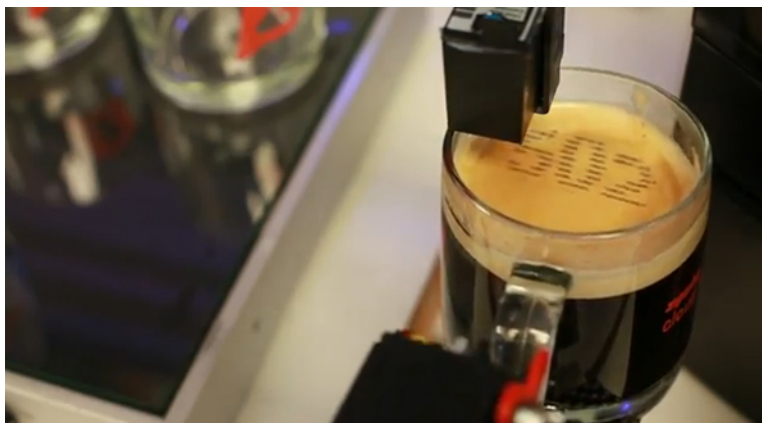
Figure 11: Textpresso, an Arduino-integrated espresso machine. The machine receives drink orders via text message and prints the order number into the foam using edible ink.
