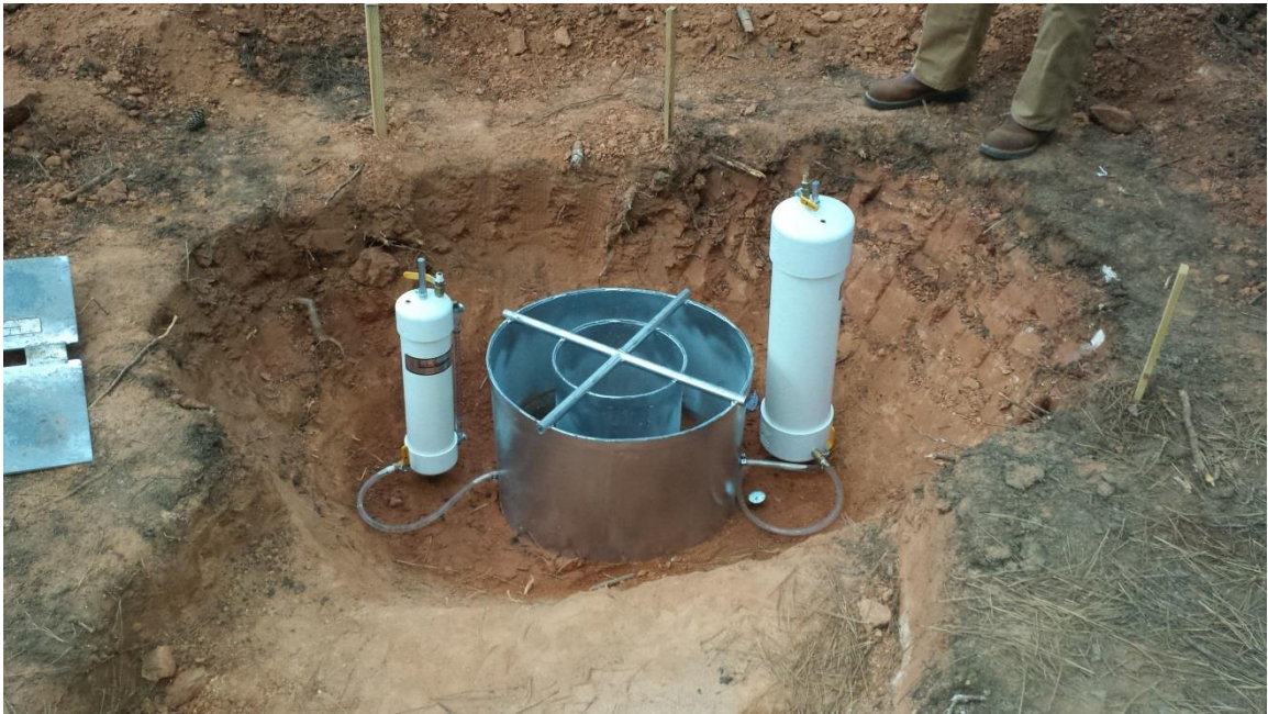
Figure 3-2 Test set up for in-situ measurement of saturated hydraulic conductivity using a double-ring infiltrometer.
