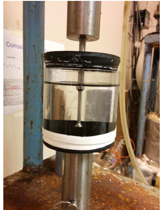
Figure 4.6: SSRT corrosion cell
