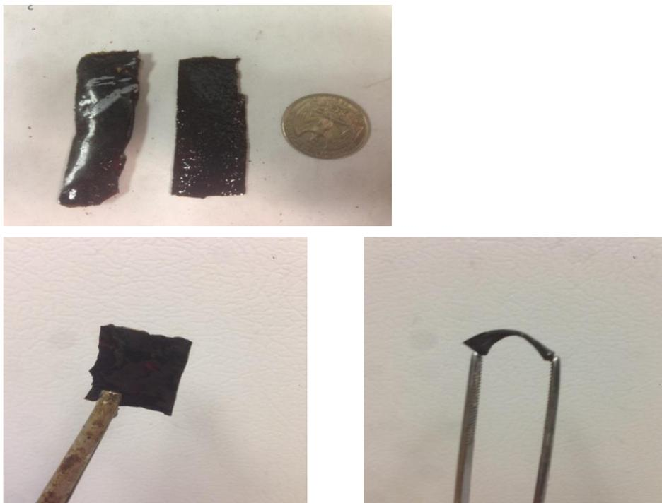
**Figure 31** Photos of polyurethane sample synthesized
