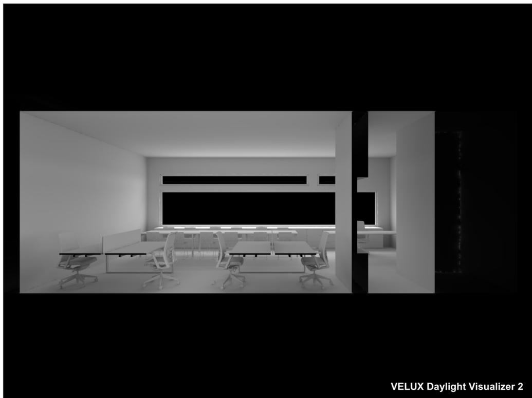
Figure 7.24. Daylighting for Atlanta Winter Noon Overcast Sky East West Section View in VELUX
