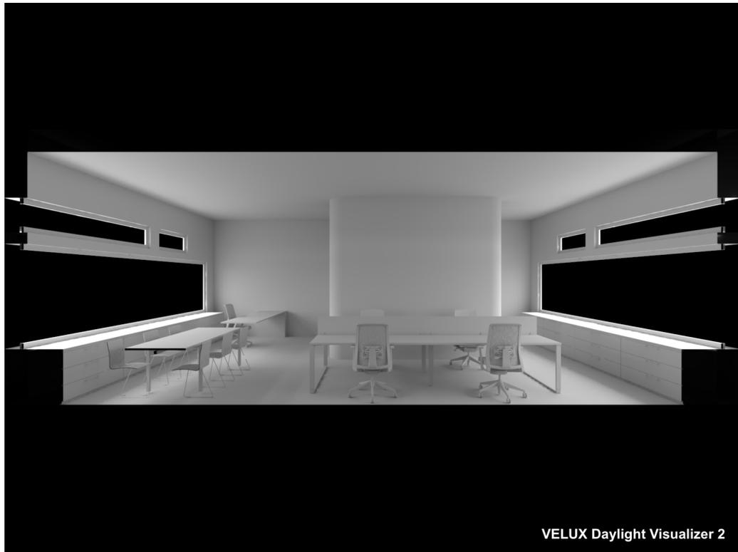
Figure 7.15. Daylighting for Atlanta Winter Noon Overcast Sky North South Section View in VELUX
