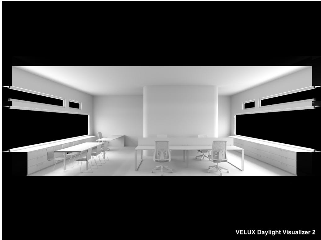
Figure 7.13. Daylighting for Atlanta Summer Noon Overcast Sky North South Section View in VELUX
