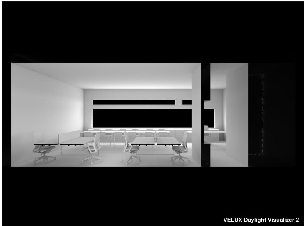
Figure 7.22. Daylighting for Atlanta Summer Noon Overcast Sky East West Section View in VELUX
