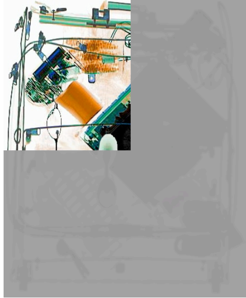
Figure 2. An example of the preview image with the remaining baggage regions displayed in reduced contrast.
