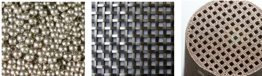
Figure 4: Examples of possible regenerator geometries.
