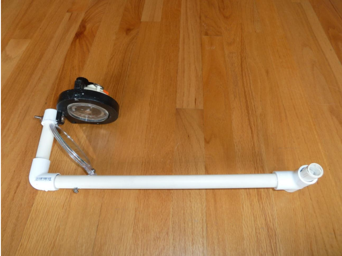
Figure 8. Mounting system for the Sekonic Marine Metre II L-164B
