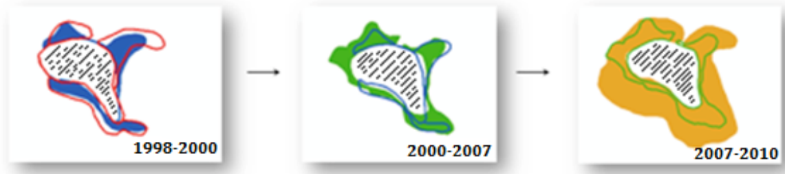
Figure 13. Example of depositional feature shape over time in CCNS. Although the depositional lobes display variety in their morphology over time, the majority of depositional lobes have a similar pattern of evolution; an initial decrease in shape metric followed by an increase in shape metric, which indicates an increase in area and a decrease in perimeter (indicative of a less complicated shape). T1 is outlined and T2 is solid, as well each year has a corresponding colour (1998=red, 2000=blue, 2005=green, and 2010=orange). The black lines represent the area of the blowout hollow.
