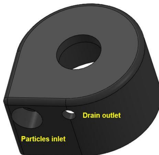
Figure 3-8: Hollow cylinder, front section
