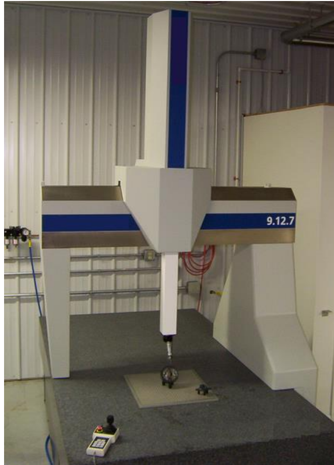
Figure 2-1: Coordinate measuring machine
