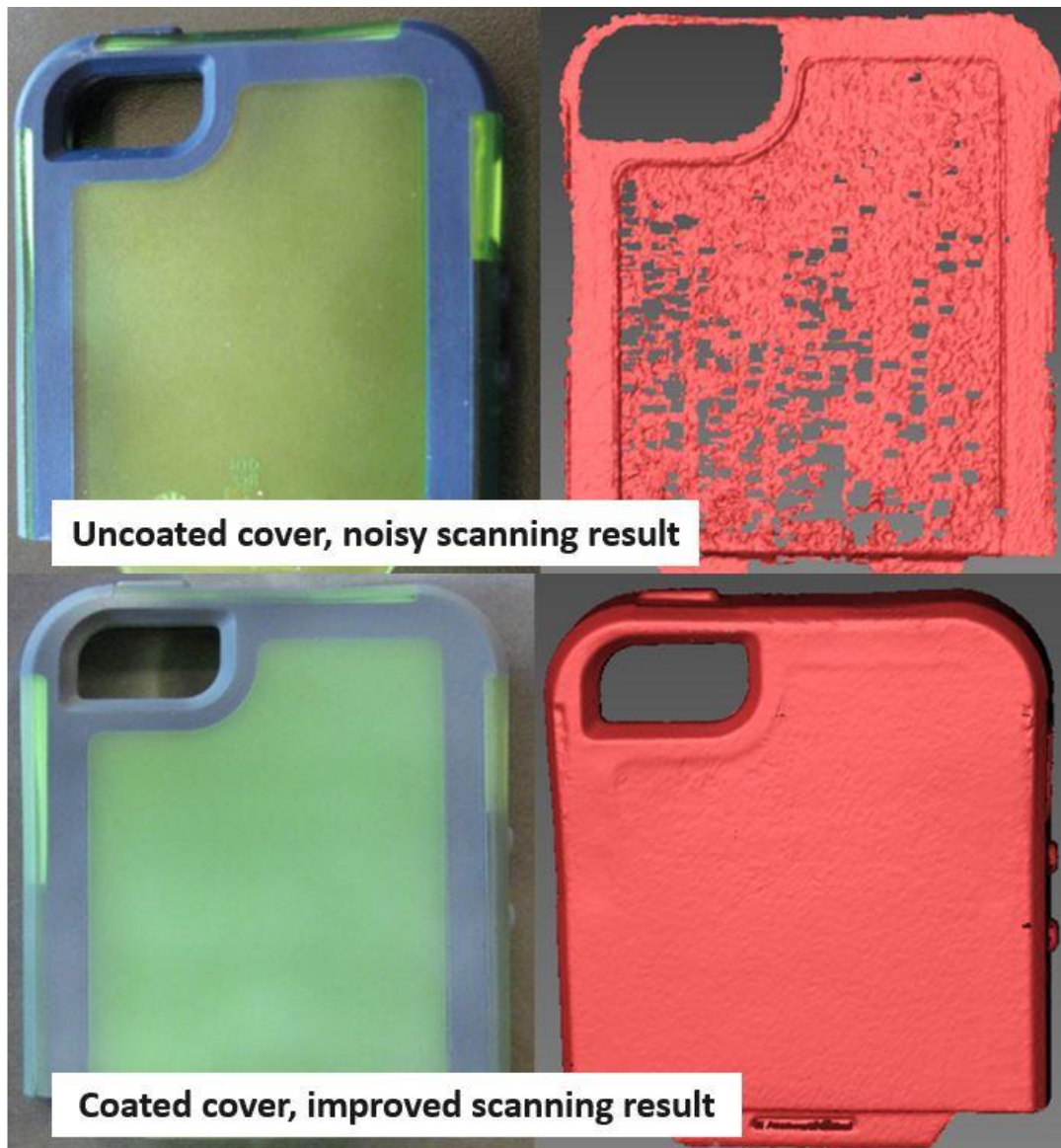
Figure 5-2: Scanning results of a translucent cell case (uncoated top and coated bottom)
