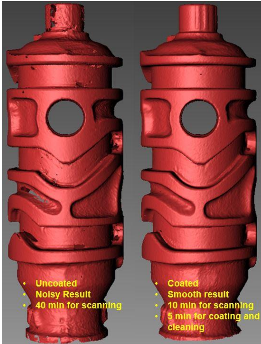
Figure 5-5: Scanning results for uncoated part (left) with around 620,000 vertices in 40 minutes and coated part (right) with around 455,000 vertices in 10 minutes
