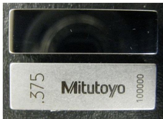
Figure 4-13: Gauge blocks as shiny samples with dark gray color
