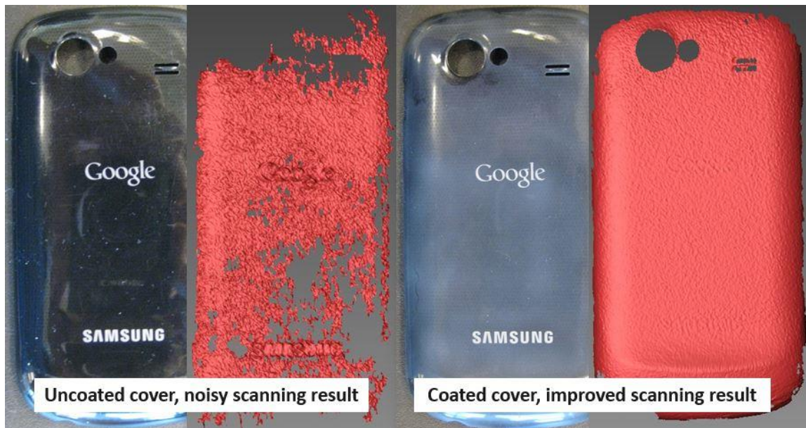
Figure 5-1: Scanning results of a black shiny cell case (uncoated left and coated right)
