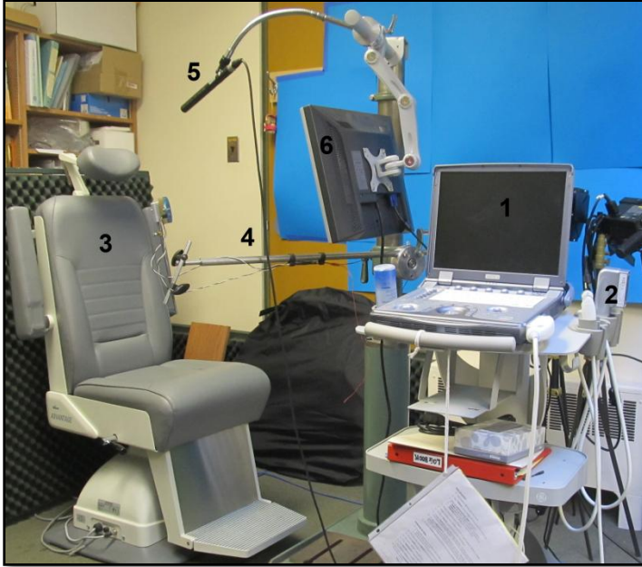
Figure 6(a). The experimental set-up: 1) portable GE Logiq E ultrasound machine; 2) ultrasound probe; 3) dental chair; 4) mechanical arm with spring-loaded probe holder; 5) microphone; 6) computer monitor mounted on the mechanical arm.
