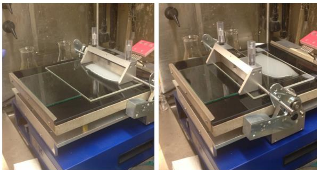
Figure 3-19. D2020-TiO 2 solution on glass plate (left) and 1 mm film after casting (right)
