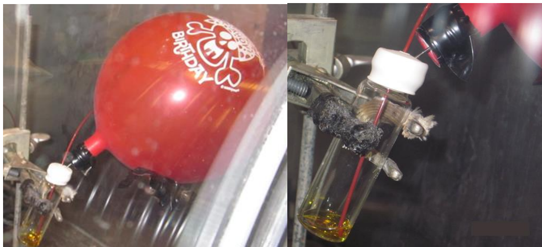
Figure 1.6. Setup for PSI-ESI-MS in the glovebox using a party balloon which provides the over-pressure of nitrogen while the solution is pushed out through the PEEK tubing to the MS.
