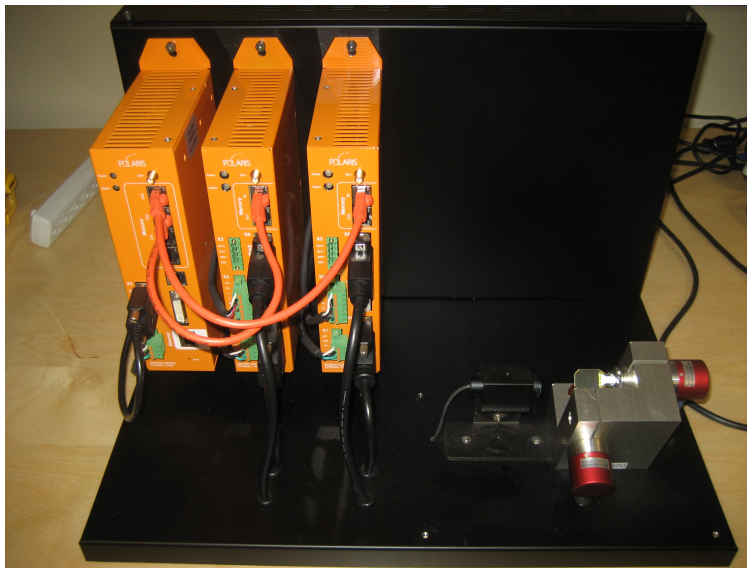
Figure 4.1: Controller, amplifiers and galvanometer set-up
