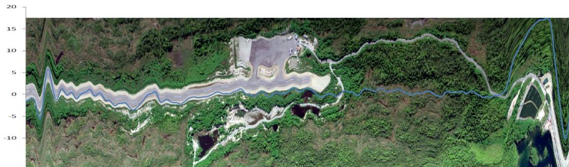
**Figure 9. Synchronized Raw Image with roll attitude plotted in blue line**
