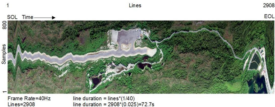
**Figure 6. Raw AIS Flightline depicted as a sequential time series**
