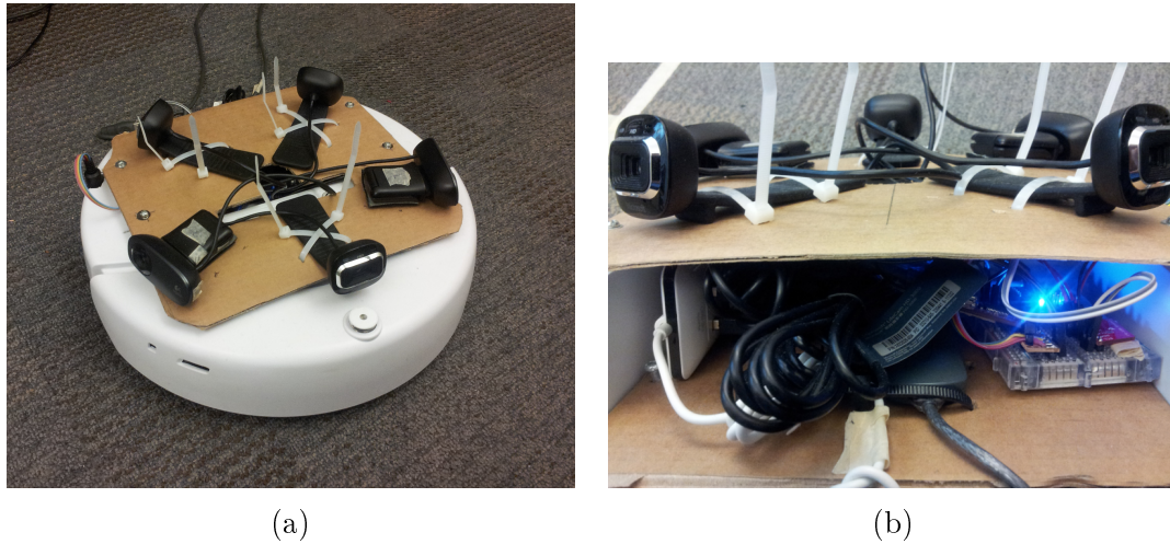
Figure 5.2: a) The iRobot Create fitted with five webcams to give the robot a near omnidirectional field of view. b) The back of the robot, showing the microcontroller and wiring.
