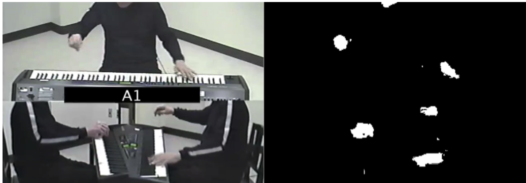
Figure 3.7: Hand tracking example. Original image is on the left and the corresponding binary skin frame on the right.
