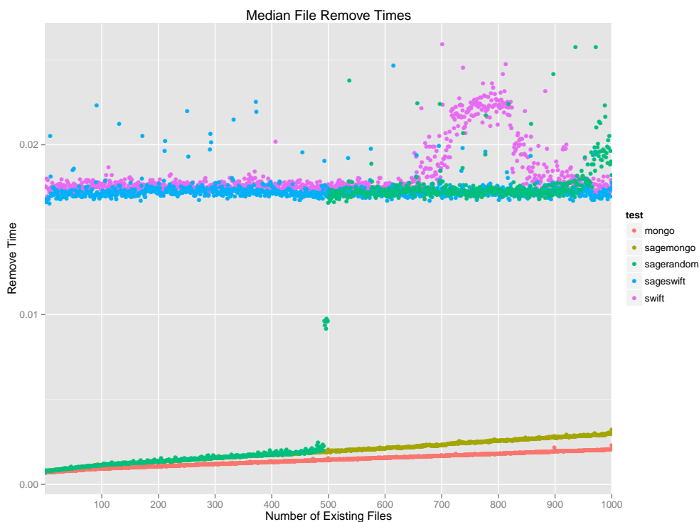
Figure 5.12: Median times to remove a file for each test run. Each test was performed 10 times with an increasing number of files already existing from 0 to 999.
