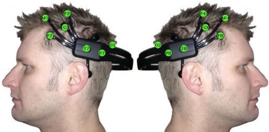
Figure 2.3: Positions of the electrodes on the Emotiv EPOC [5].
