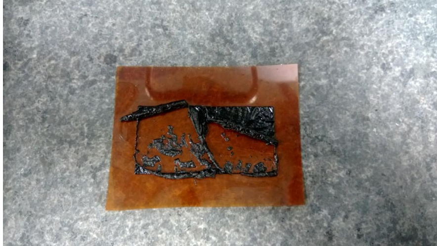
Figure 3-7 Nanocyl 1% (w/v) after ~5 seconds of the exposure at 400 W/in 2 .
