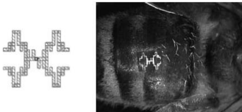
Figure 2-11 Example of awkward, conformal antenna on a honeybee's abdomen; from Ref [11].
