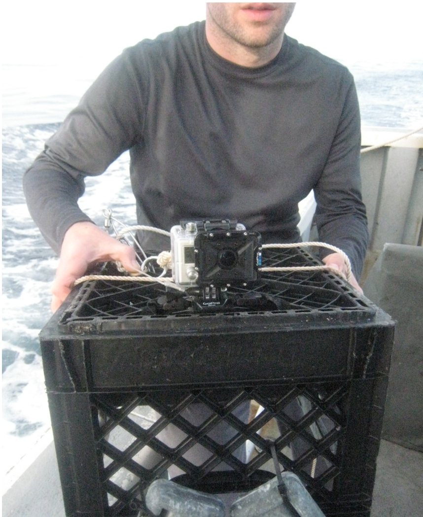
Figure 3. Custom-made camera stand: a weighted milk crate mounted with a GoPro™ camera.
