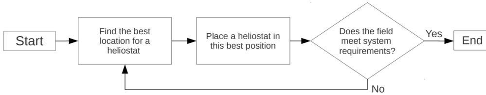
**Figure 2.3:** Field growth method procedure
