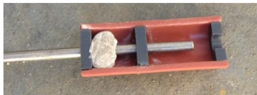
Figure 4.8: Photo of the receptacle for the deluge water thermocouples
